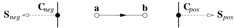
Figure 8.3: The physical interpretation of the value of \lambda_a . Face neg yields a negative value of \lambda_a , face pos yields a value of \lambda_a greater than 1.
