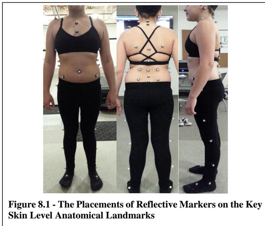
The Vicon Nexus software system (Oxford, U.K) and its cameras collected three-dimensional (3D) Cartesian coordinate geometric data from the markers (Figure 8.2 (a)). Each capture time lasted about 10 seconds. The values for each 3DSP were calculated from the geometric data obtained from the reflective markers using equations programmed in bespoke Lua script modules in Motek (D-flow) software (Amsterdam, Netherlands) (Figure 8.2 (b)).
