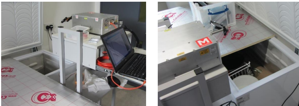
Figure 4.21. Experimental setup for the small sample runs of ice imaging. The two photographs depict the Firefly IR Imager next to the Labcold freezer imaging the ice sample located inside the freezer.
