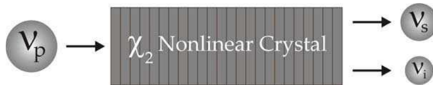
Figure 2.17. Schematic of the parametric frequency down-conversion process where high energy pump photon is split into lower energy signal and idler photons [81].
