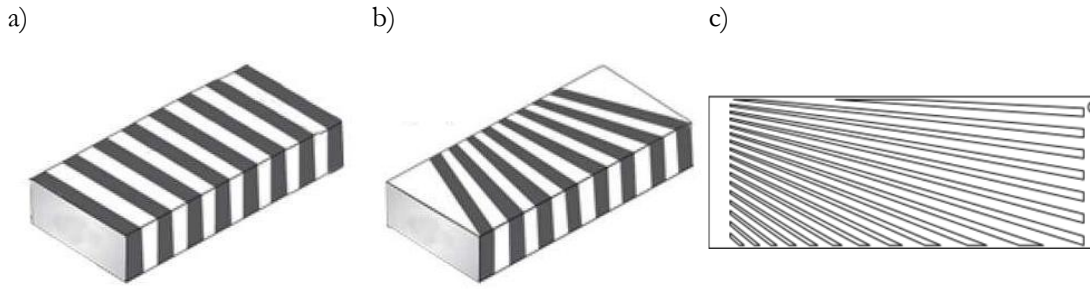
Figure 2.19. Periodically poled nonlinear crystal structure with a) single, b) fan-out [81] and c) slanted fan-out [85] grating periods.
