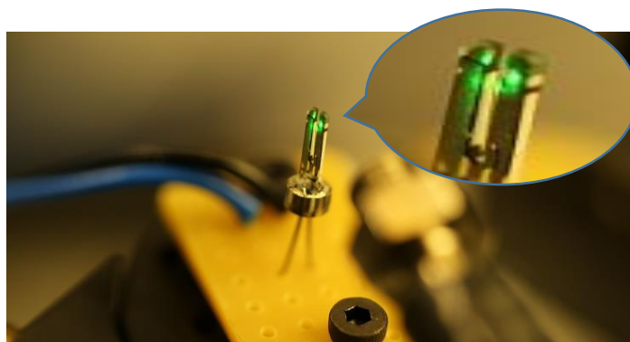
Figure 5.48. Bare QTF with laser on. The green light visible on the prongs of the QTF results from the parasitic doubling of the 1064nm pump.
