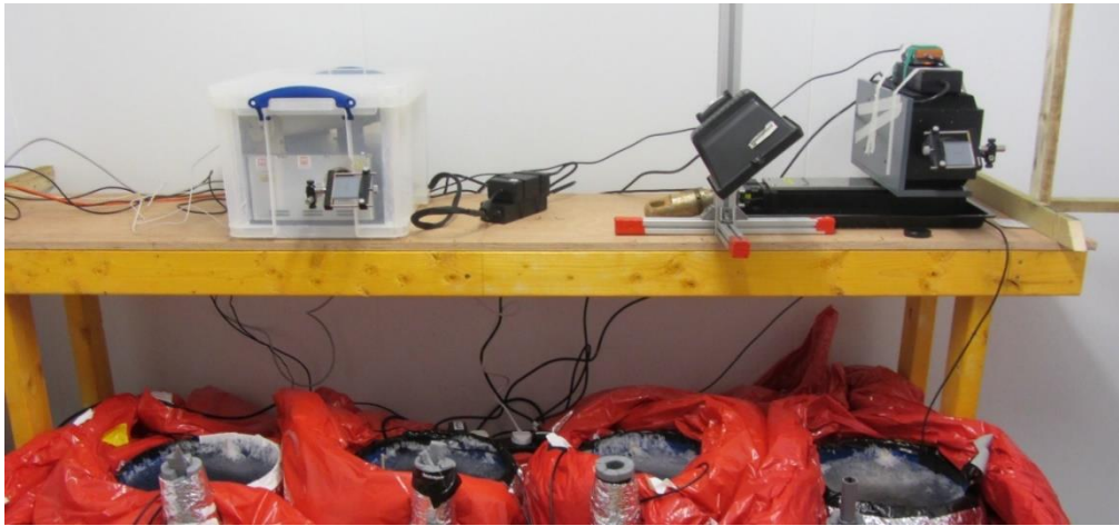
Figure 4.3. Firefly IR Imager in thermal enclosure (on left) and Red Eye 1.7 camera mounted on the translation stage with halogen illumination (on right) in the testing setup.
