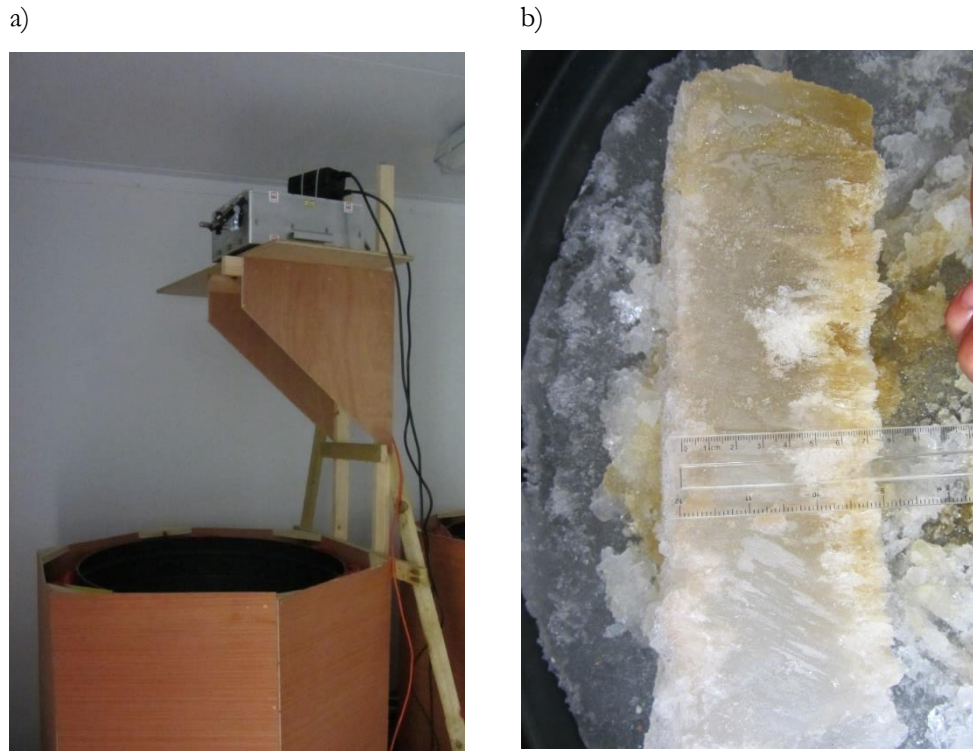
Figure 4.2. Scanning setup with the Firefly IR Imager above the container with ice (a); the ice block of approximately 80 mm thickness cut after the imaging (b).
