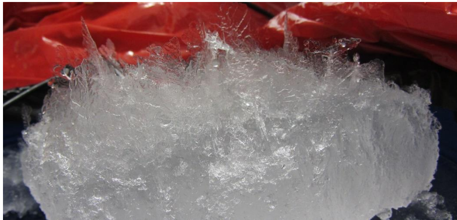
Figure 4.12. Ice formation stuck to the bottom surface of the main ice layer – view of the bottom of the ice block cut out from the contained after imaging.
