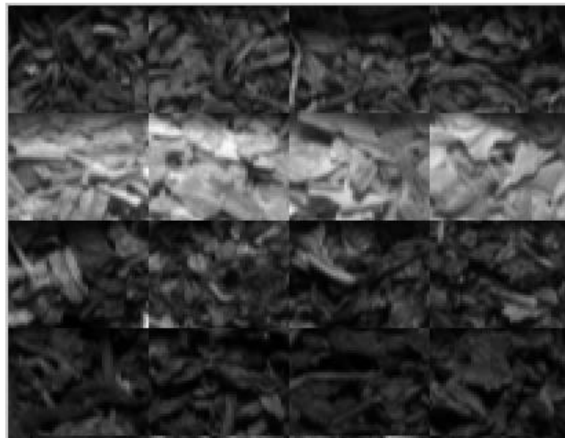
Figure 2.8. Single intensity image from the hyperspectral data used in this example. Image represents 4 different types of tea leaves (rows) with 4 snapshots per each type (columns) combined in one picture.
