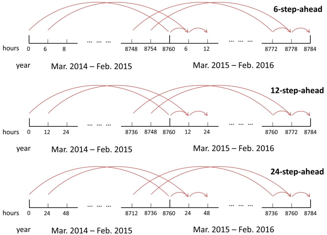
**Figure 5-9:** The load demand forecasting processes of 6-step-ahead, 12-step-ahead and 24-step-ahead forecast
