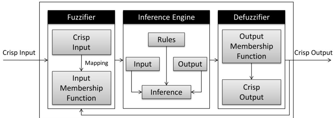
**Figure 3-2:** Structure of a fuzzy logic system
