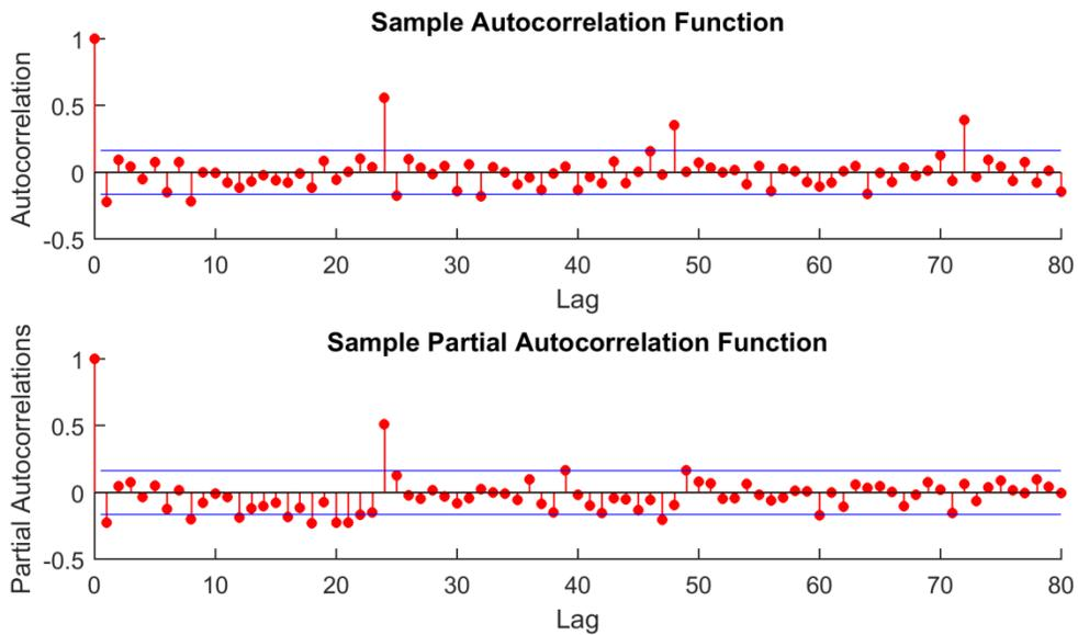
**Figure 3-13:** ACF and PACF of the load demand data after 1<sup>st</sup> and 24<sup>th</sup> differencing
