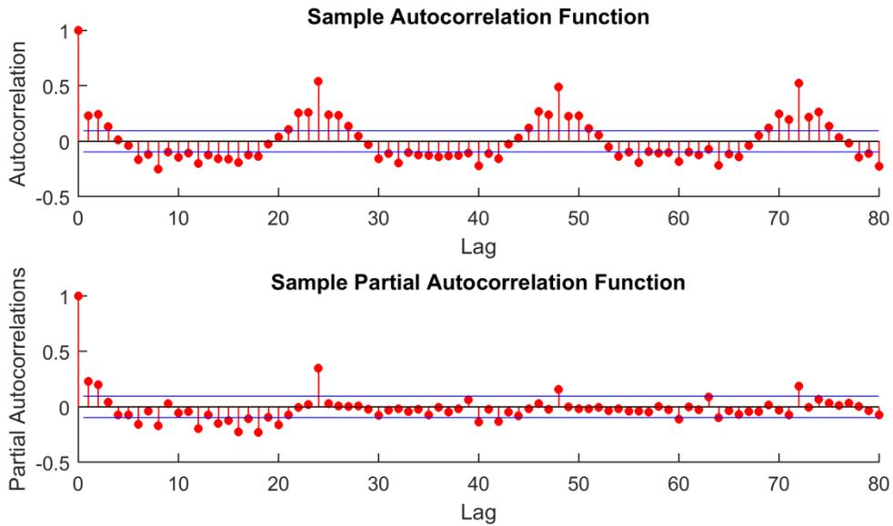
**Figure 3-12:** ACF and PACF of the load demand data after 1<sup>st</sup> differencing
