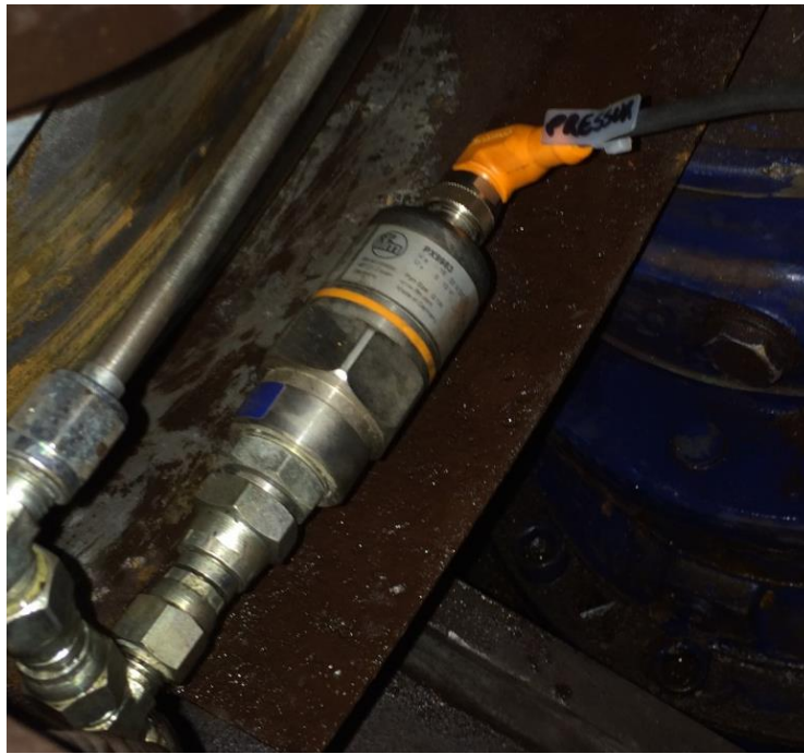
Figure 11: Pressure sensor used to measure the oil pressure applied to the emergency brake [55]
