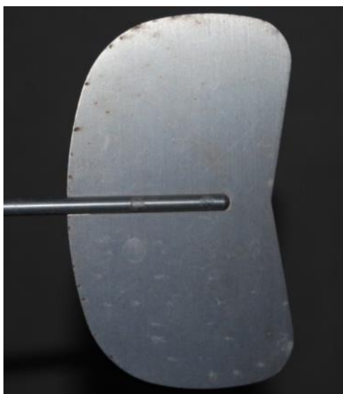
Figure 19: Wind vane following suspected lightning strike
