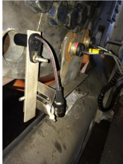
Figure 30: Hall-Effect Sensor for measuring rotational speed
