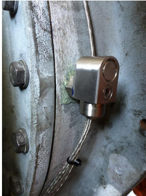
Figure 9: Accelerometer mounted on main bearing
