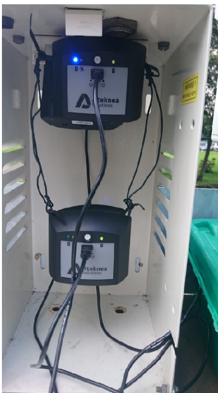
Figure 2: Deployment of the four LEO instruments (two instruments located back to back) in a passively ventilated enclosure on the roof of Townhead automatic monitoring station.
