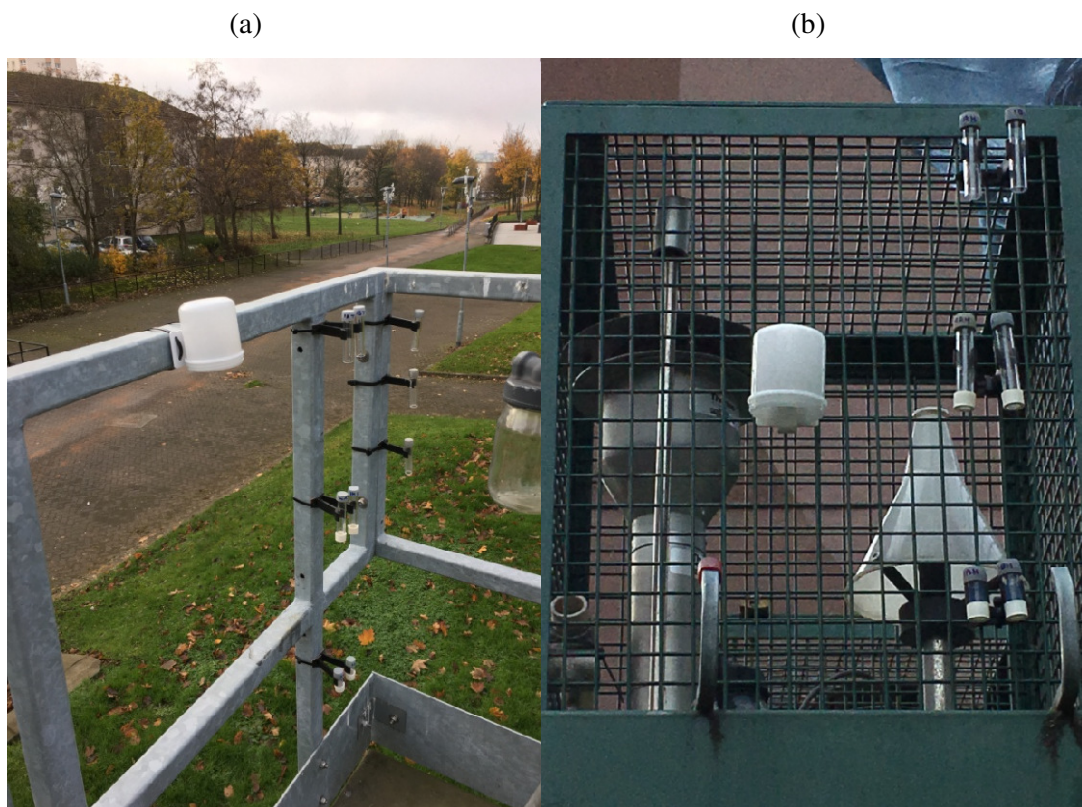
Figure 1: Deployment of the passive diffusion samplers at (a) Townhead and (b) High Street. Townhead samplers were mounted on a railing on the roof of the site located ~1 m from the analyser inlets, while High Street samplers were located on the cage on the roof of the site which also contained the analyser inlets.
