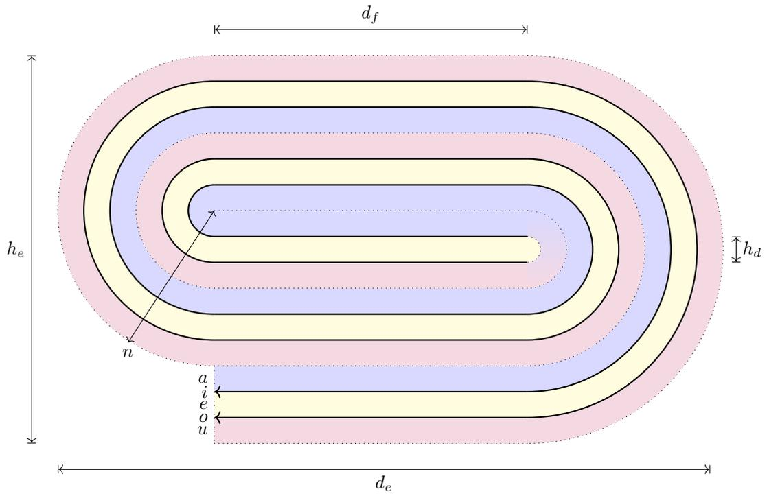
Figure 6.4: A concentric element with 3 dielectric layers
