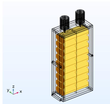
Figure 5.12: A 9-winding, 40-turn model
