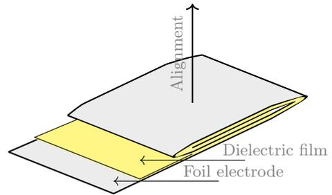
Figure 2.2: A simple winding
