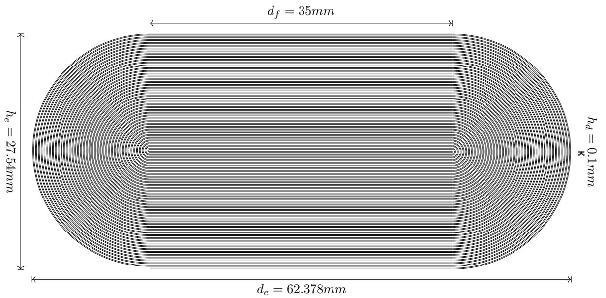
Figure 6.5: A second concentric element with 3 dielectric layers
