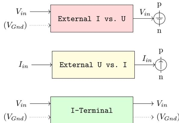
Figure 3.5: Nodes to couple geometrical (left) to Electric Circuit (right) physics
