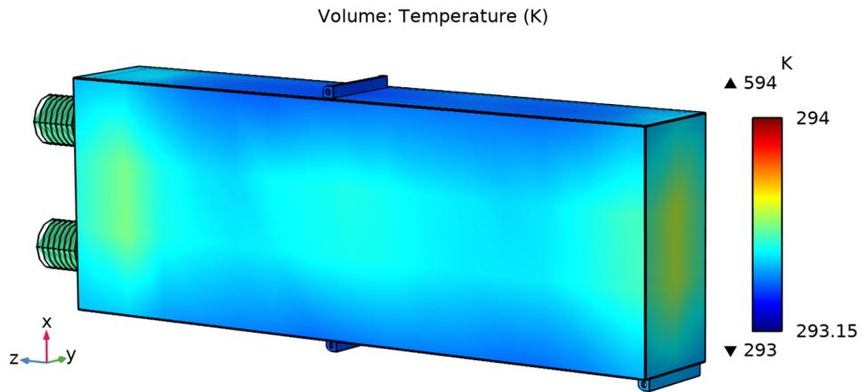
Figure 5.6: Point heat source on a penultimate foil
