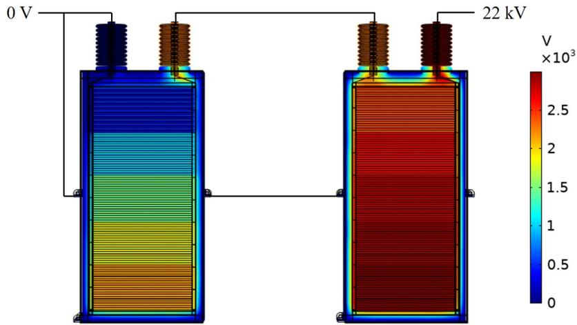
Figure 4.22: Voltage shared by units connected to a rack (left) and to 22 kV (right)
