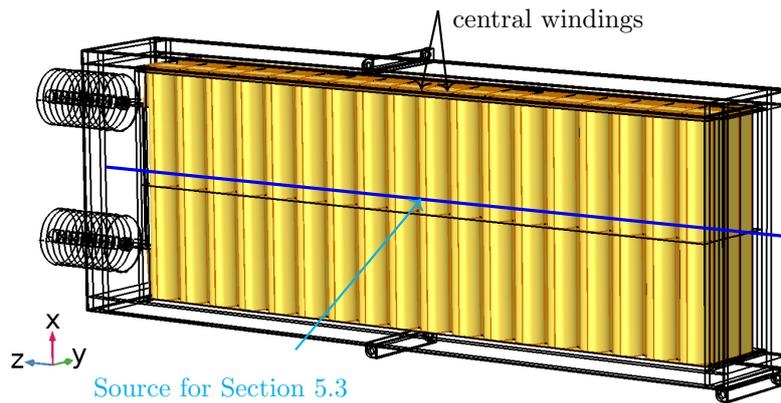
(c) Foils aligned to the Z axis
