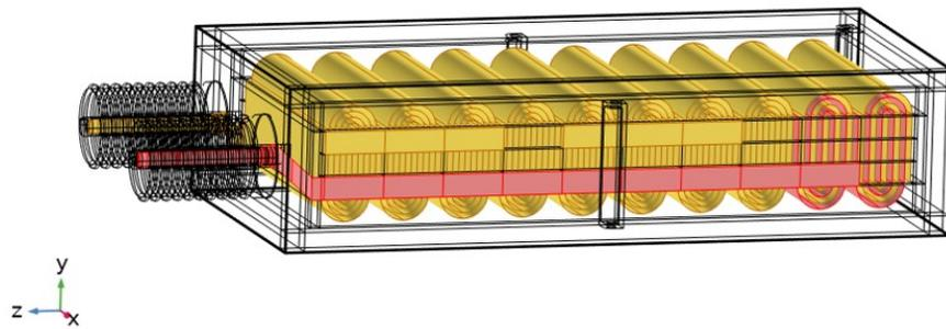
Figure 4.6: Unit with 10 windings connected as 5 series element groups
