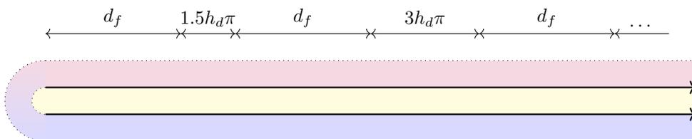
Figure 6.6: A flattened concentric element with 3 dielectric layers
