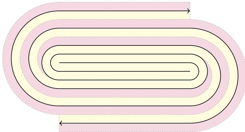
Figure 6.13: A graded counterroll element with 3 dielectric layers
