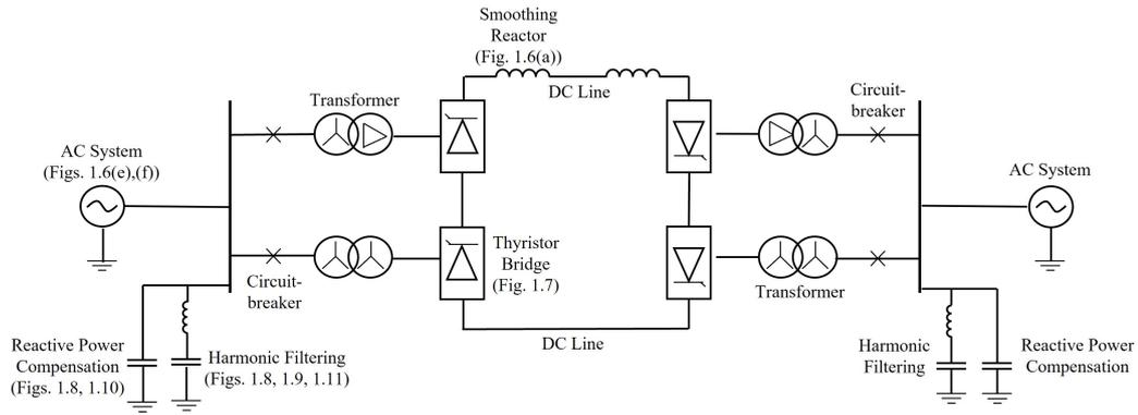
Figure 1.3: Line diagram of an LCC HVDC link [8]
