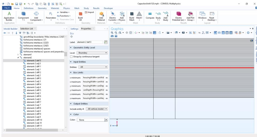
Figure 3.9: Selecting an innermost winding boundary with a box selection
