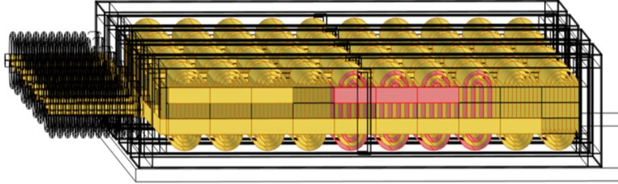
Figure 4.20: Foils in a capacitor unit with 5 series groups of 2 elements each
