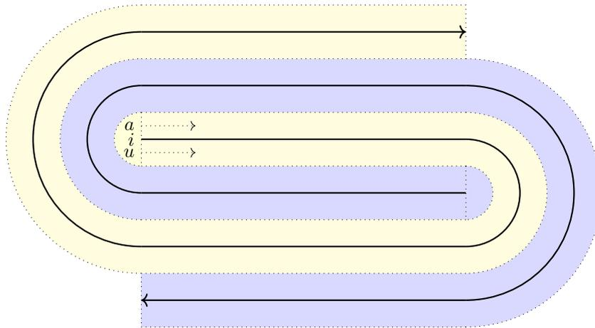
Figure 6.7: A counterroll element with 2 dielectric layers
