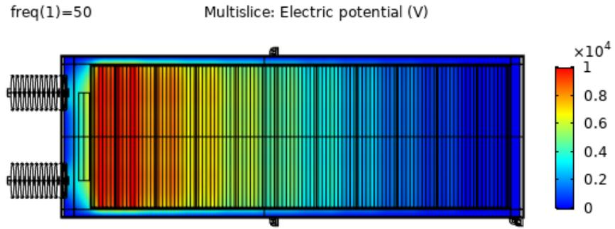
(a) Voltage over an XZ-plane cross-section
