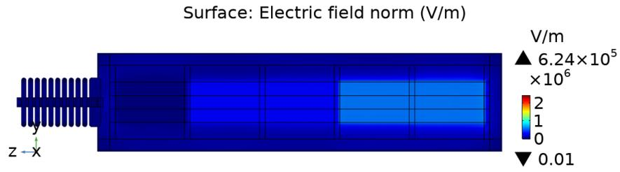
(a) A cut plane in YZ showing the distribution of electric field between adjacent interleaved windings
