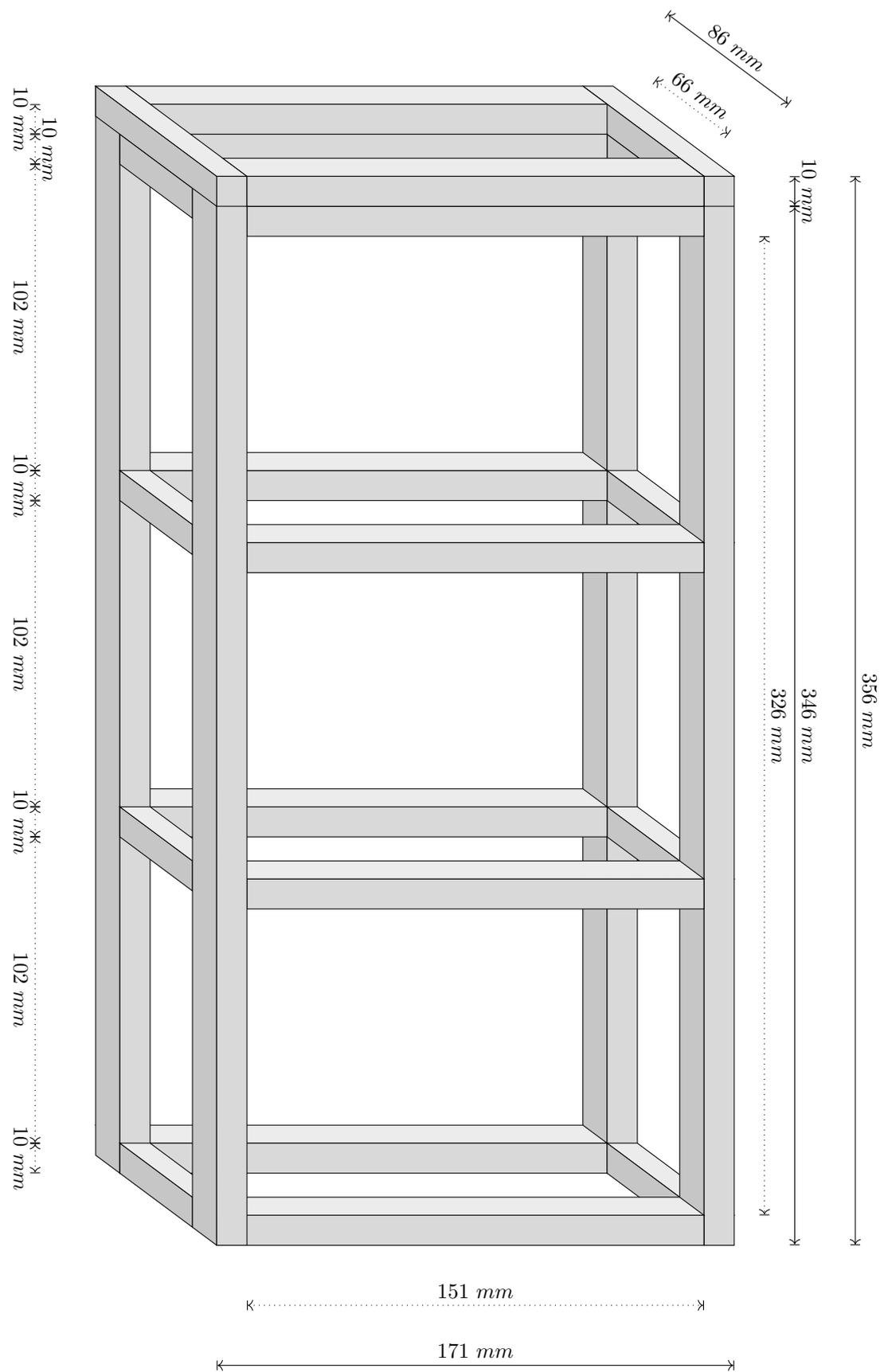
Figure 6.1: Frame for a scale model
