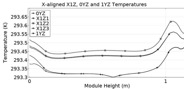
(c) Temperature along X1Z, 0YZ, and 1YZ cut lines for heat on a tab connector
