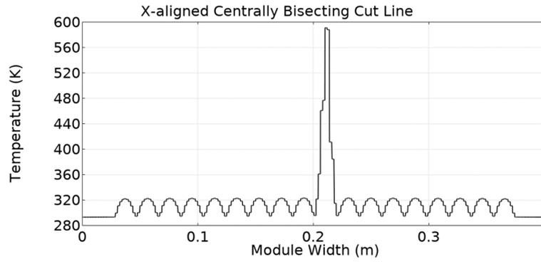
(a) Temperature along a centrally bisecting cut line for a central heat source
