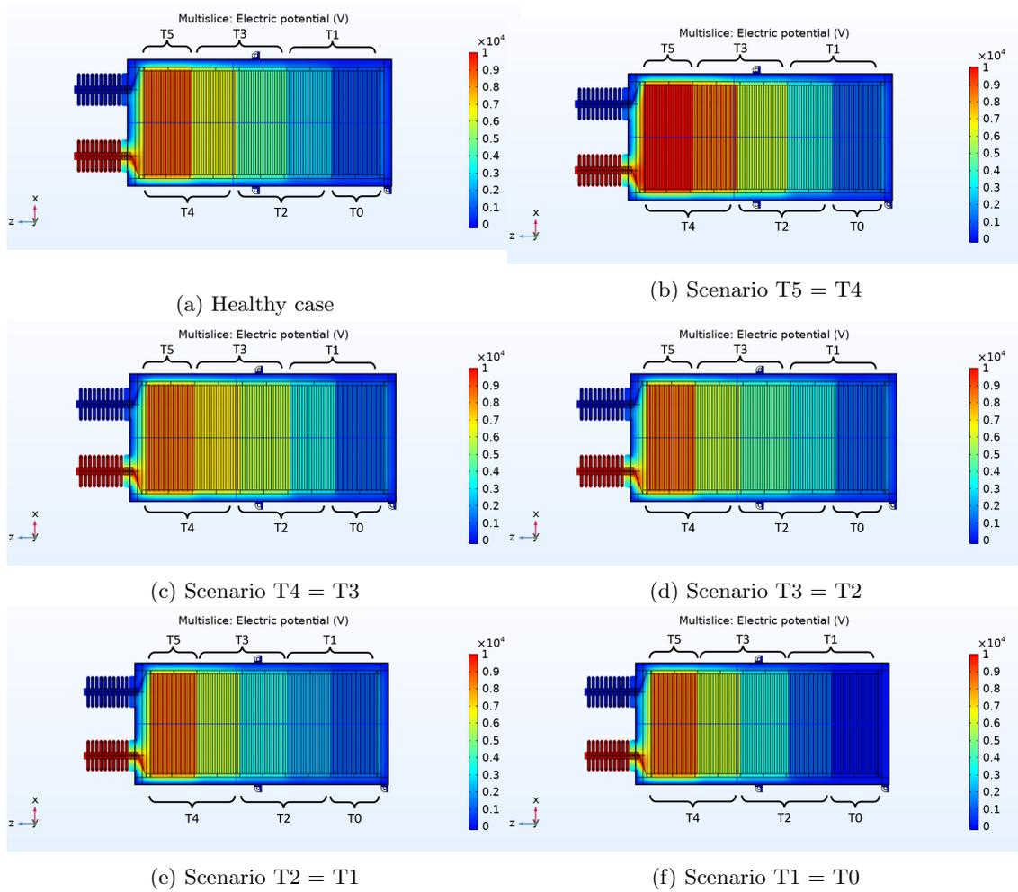
Figure 4.10: Electric potential in an XZ cut plane
