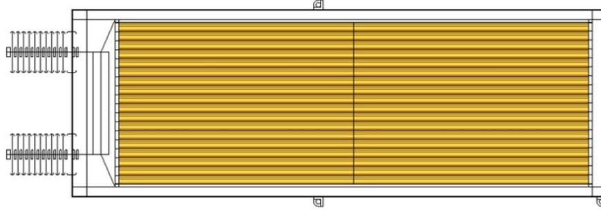
Figure 5.1: A capacitor model with foils aligned to the X-axis
