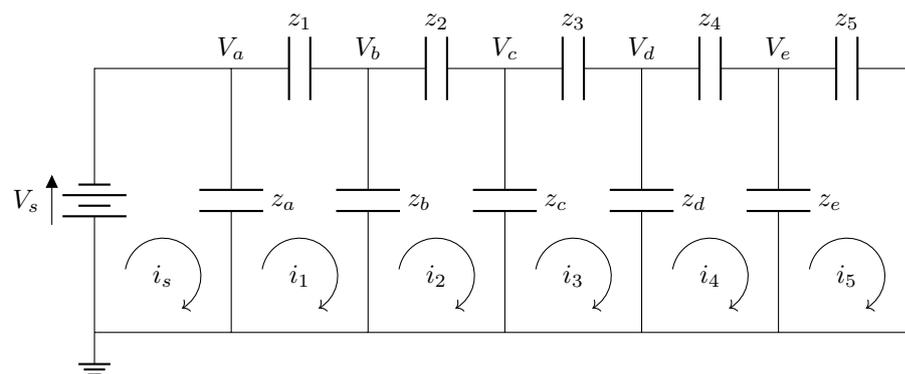
Figure 4.7: Circuit diagram equivalent to the unit in Figure 4.6.
