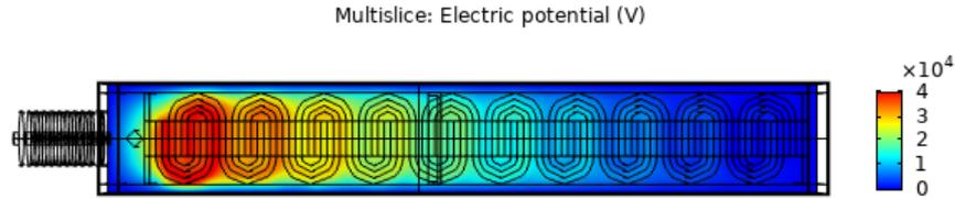
(b) Voltage over a YZ-plane cross-section
