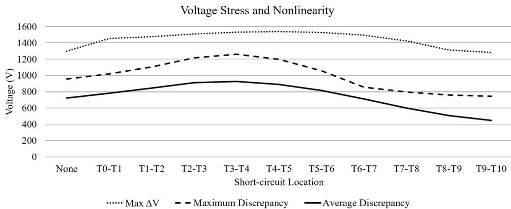
Figure 4.4: Voltage stresses between foils and deviation from a straight line
