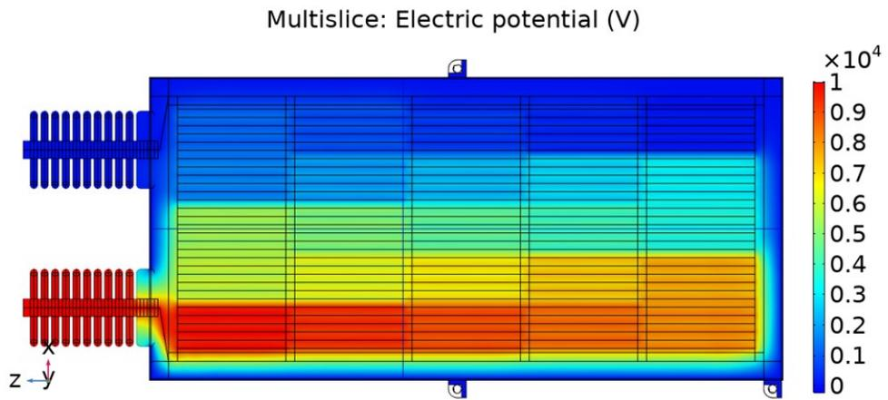
Figure 4.14: A cut plane shows voltage to increase within each interleaved winding
