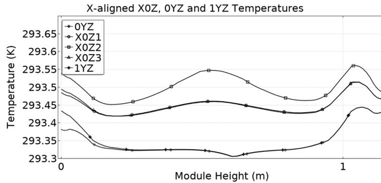
(b) Temperature along X0Z, 0YZ, and 1YZ cut lines for a penultimate foil heat source
