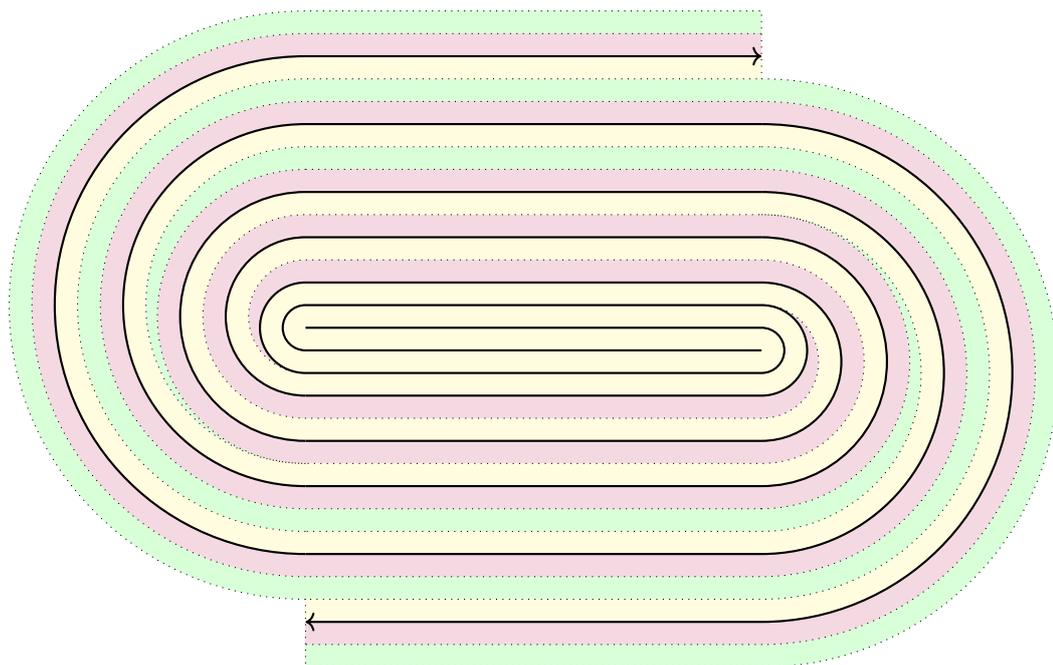
Figure 6.15: A graded counterroll element with 5 dielectric layers
