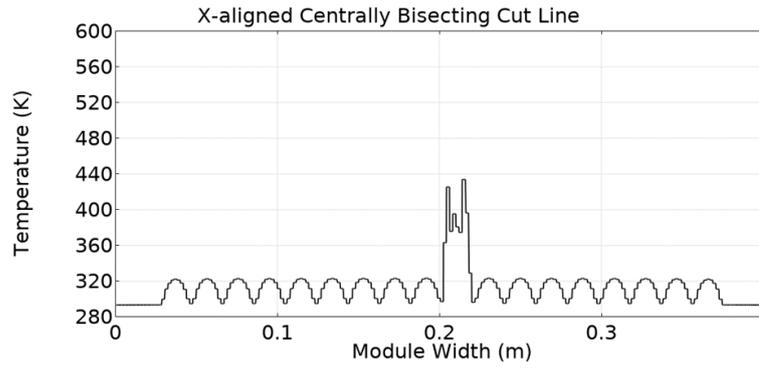
(a) Temperature along a centrally bisecting cut line for a penultimate foil heat source
