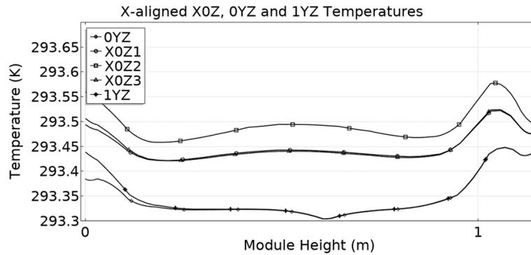
(b) Temperature along X0Z, 0YZ, and 1YZ cut lines for a central heat source
