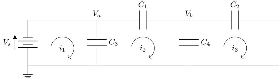
Figure 4.5: A simplified equivalent circuit with stray capacitances  $C_3$  and  $C_4$
