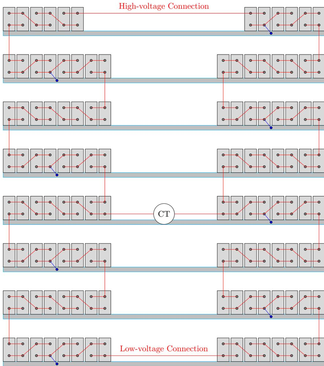
Figure 7.1: Jumper (red), rack tie (blue), and CT connections for both sides of a large bank
