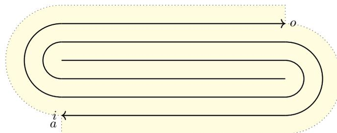
Figure 6.9: A counterroll element with 1 dielectric layer
