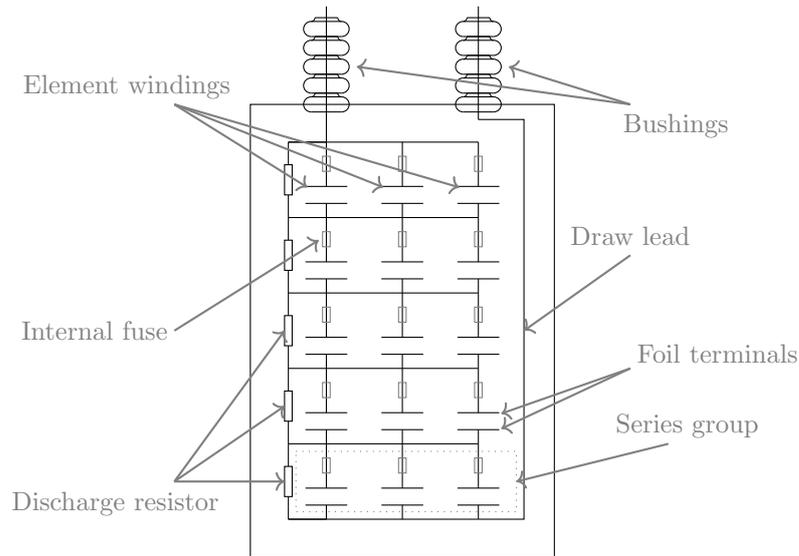
Figure 2.1: A capacitor unit line diagram [28]
