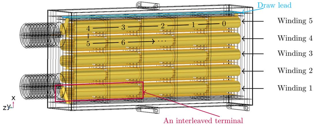
Figure 4.11: A unit with interleaved foil windings in yellow and numbered elements
