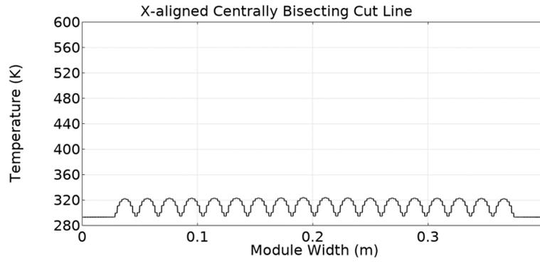
(a) Temperature along a centrally bisecting cut line for heat on a tab connector
