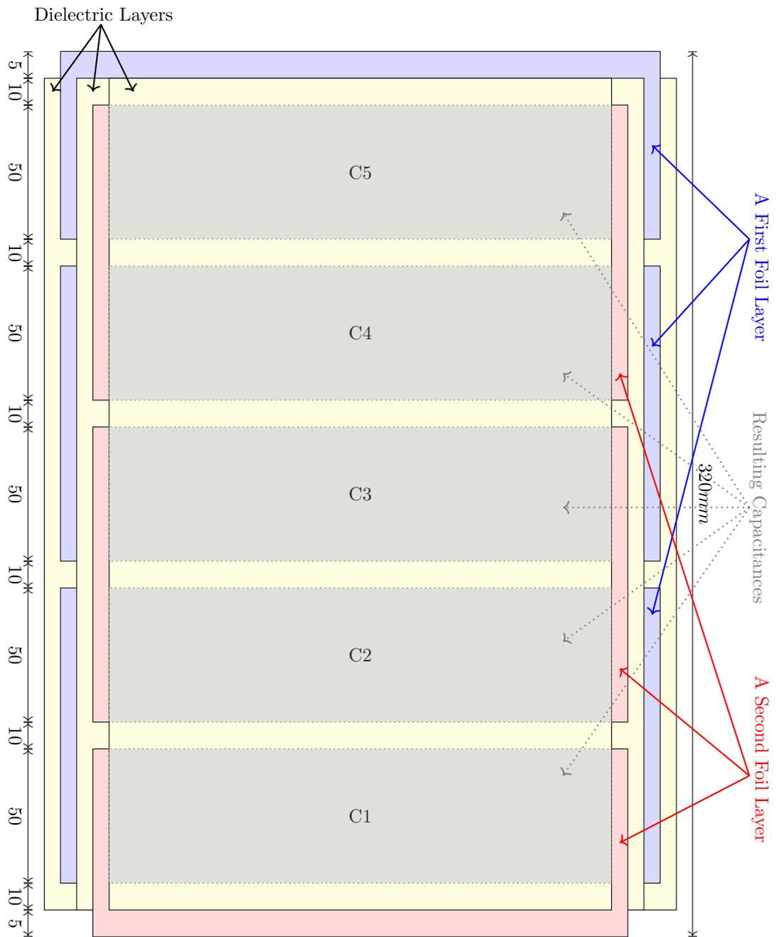
Figure 2.3: Design of interleaved windings
