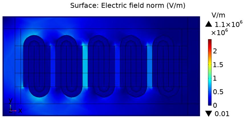
(a) A cut plane in XY at Z2 showing electric field effects at the centre of 5 elements
