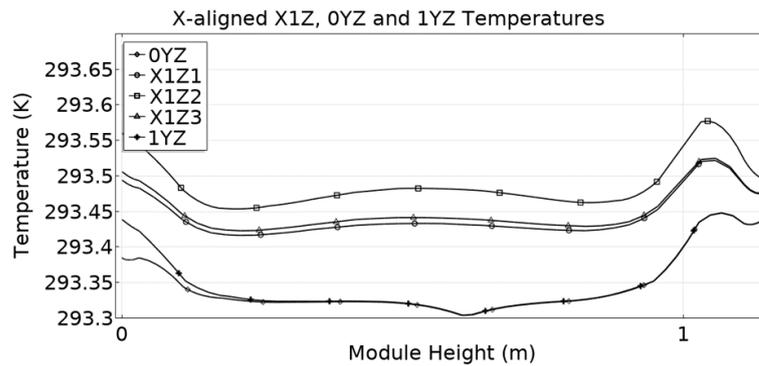
(c) Temperature along X1Z, 0YZ, and 1YZ cut lines for a central heat source
