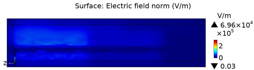
(c) A cut plane in YZ showing minimal electric field between a draw lead and housing
