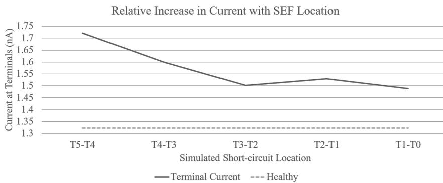
Figure 4.9: Relative change in terminal current for each fault location
