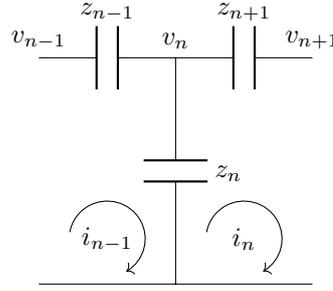
Figure 4.8: Stray capacitance in the general case
