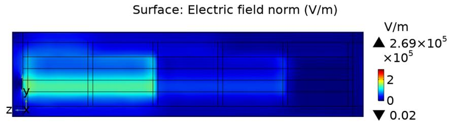
(b) A cut plane in YZ showing heightened electric field between a winding and a draw lead
