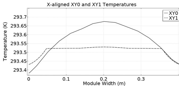
(d) Temperature along XY0 and XY1 cut lines for a penultimate foil heat source
