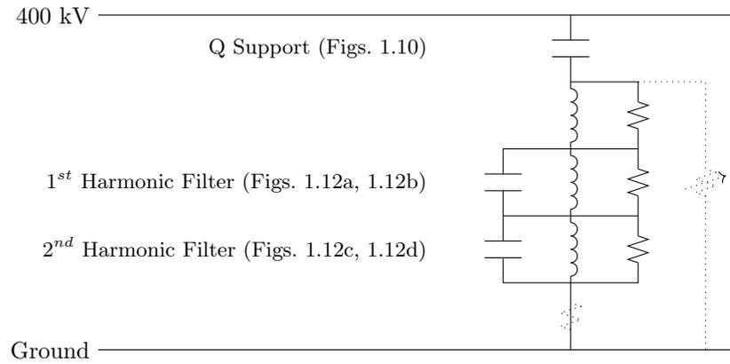
Figure 1.5: A filter bay line diagram (p108, [9])
