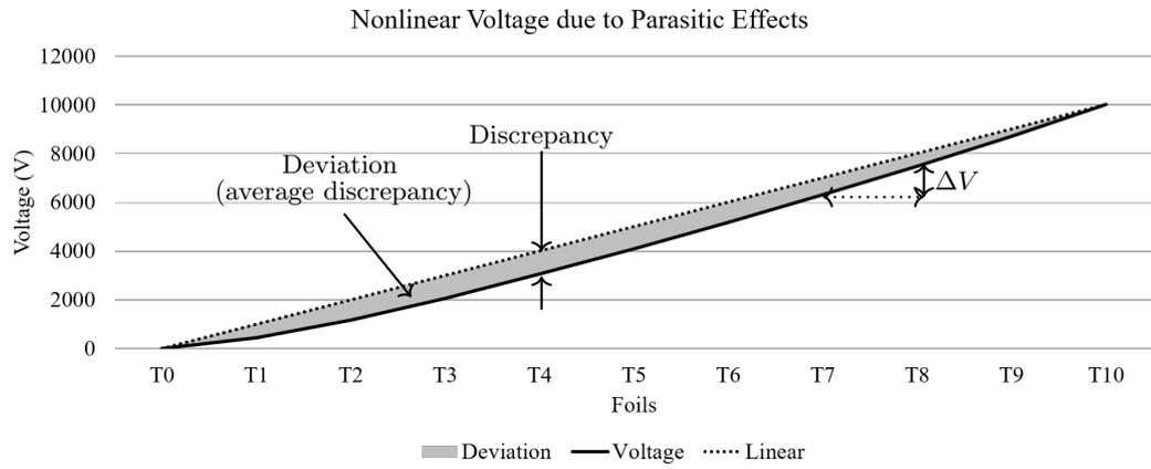
Figure 4.3: Nonlinear voltage due to parasitic effects
