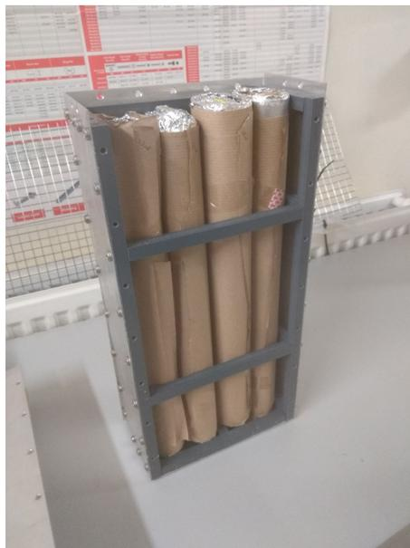
Figure 6.26: Windings in housing
