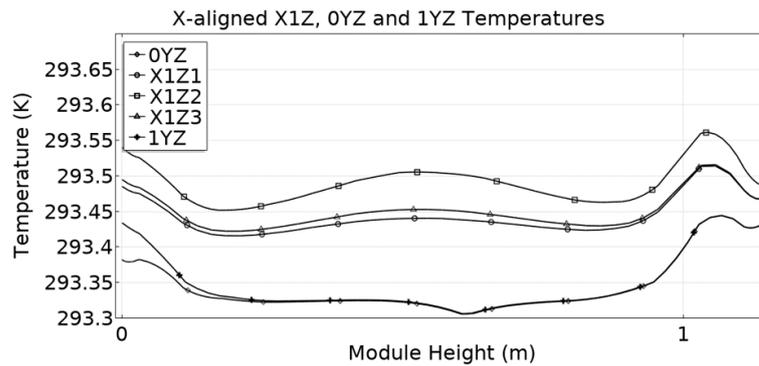
(c) Temperature along X1Z, 0YZ, and 1YZ cut lines for a penultimate foil heat source
