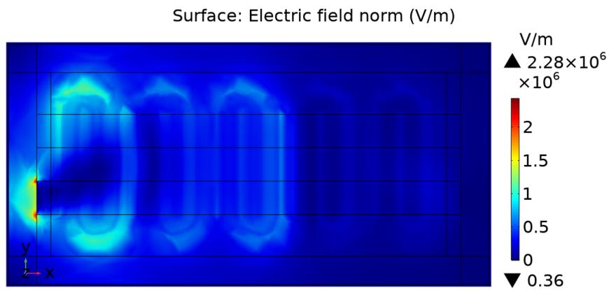
(c) A cut plane in XY at ZMax showing electric field effects near unit bushings
