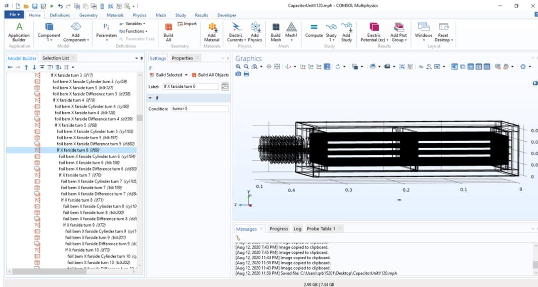
Figure 3.6: A sequence of repeated conditional geometry nodes
