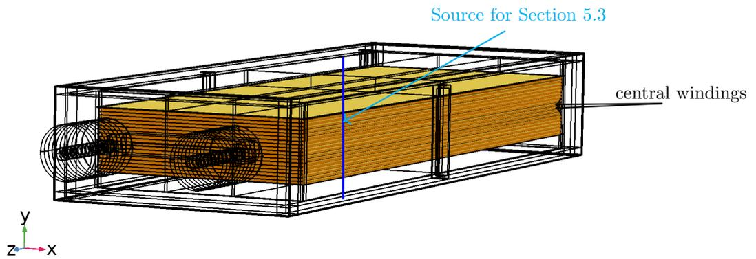
(b) Foils aligned to the Y axis (rotated to show winding turns)
