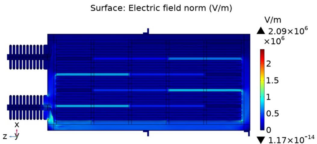
Figure 4.15: An XZ cut plane shows where field stresses arise between adjacent windings
