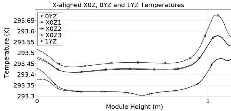
(b) Temperature along X0Z, 0YZ, and 1YZ cut lines for heat on a tab connector
