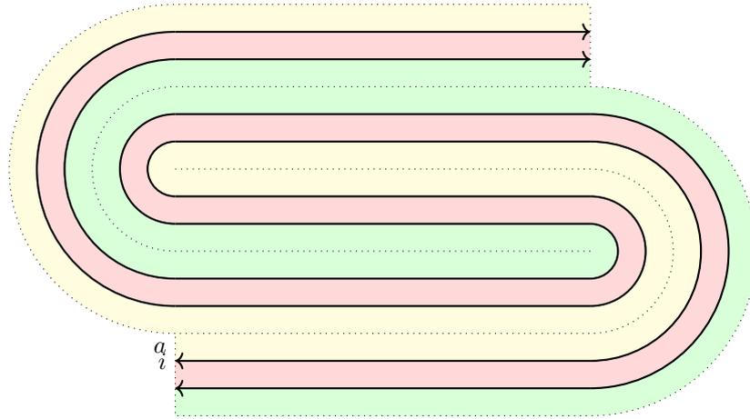
Figure 6.11: A continued element with 3 dielectric layers
