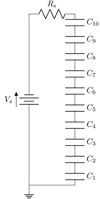
Figure 3.4: Coupling an electric circuit interface with a 10-element model
