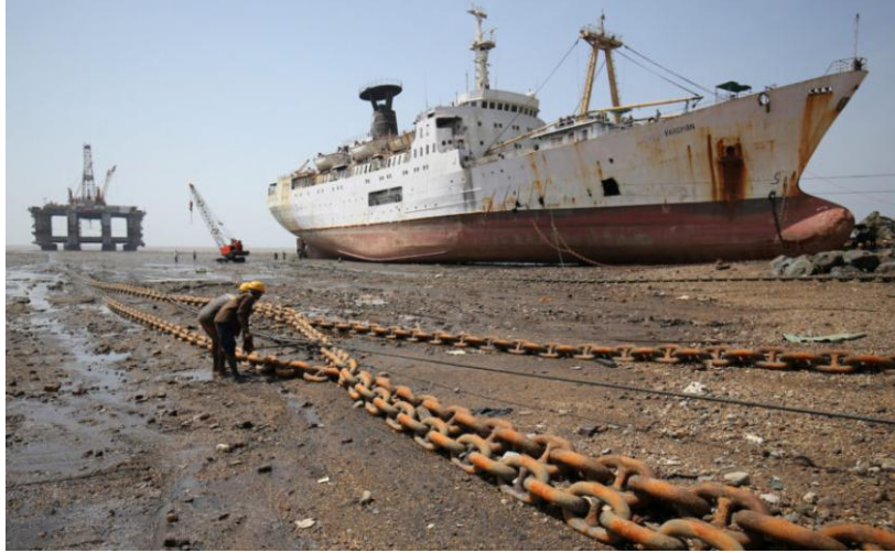
Figure 2. 6: Beaching method in Indian ship recycling yard
