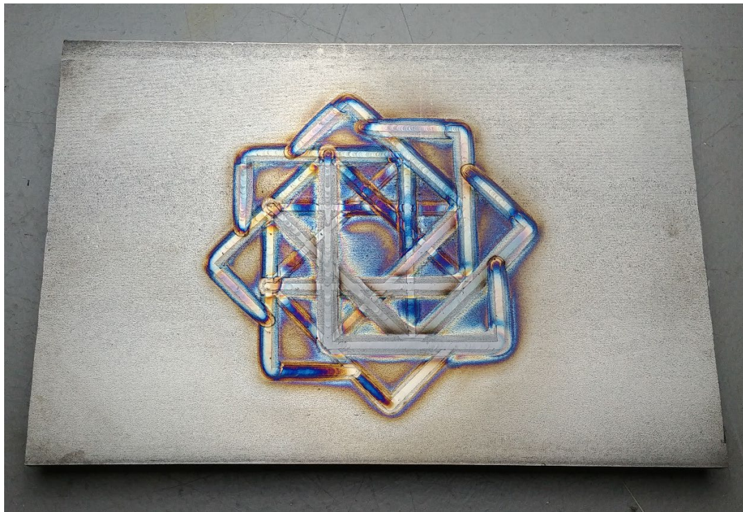
Figure 3.8 Complex pattern created through autogenous GTAW welding for the Images of Research Competition.
