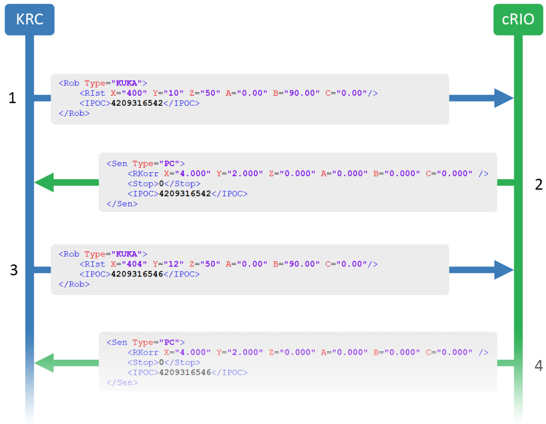
Figure 3.5 RSI communication between KRC and cRIO via XML string messages.
