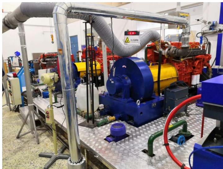
Figure 4.1 YC6K DF engine testbed
