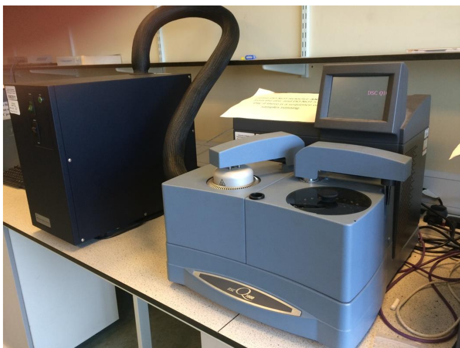
Figure 2.19 TA instruments Q1000 DSC
