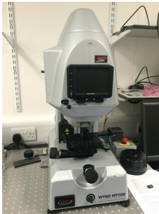
Figure 2.21 Veeco NT1100 optical profilometer
