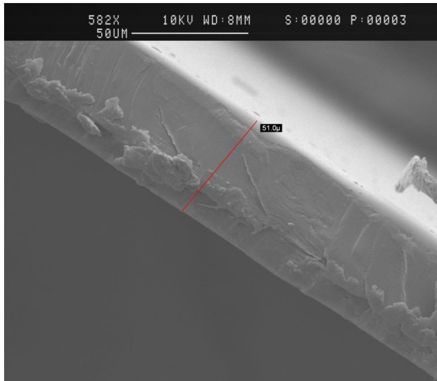
Figure 3.16 Cross-section of Untreated Mylar® A sample
