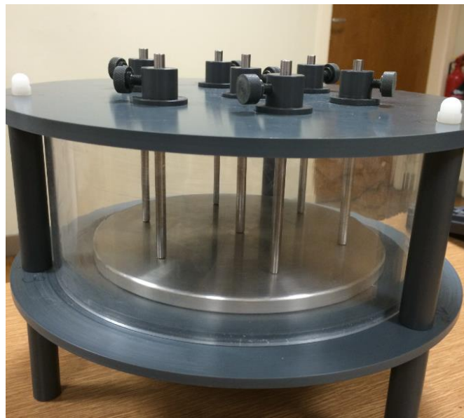
Figure 2.2 Sample holder for multiple-samples PD test
