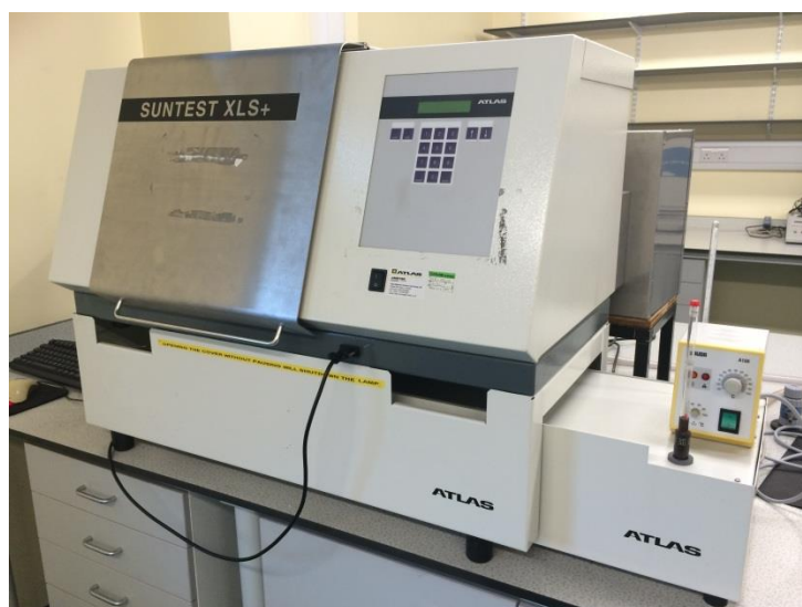
Figure 2.5 Suntest XLS+ weatherometer
