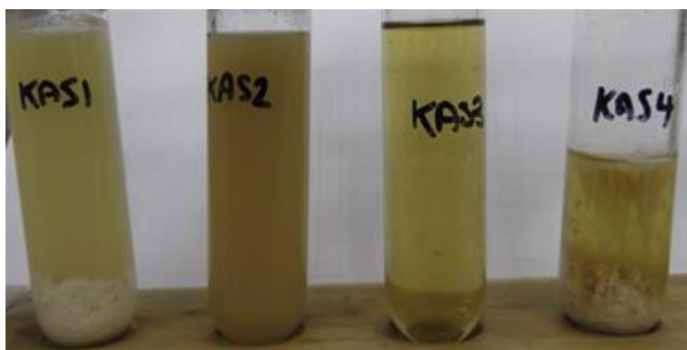
Figure 2.16: Photograph taken at the end of the reaction of KA51, KA52, KA53 and KA54 (left to right, solvents are water, ethanol, methanol and water). KA54 was designed to be a more concentrated experiment of KA51.
