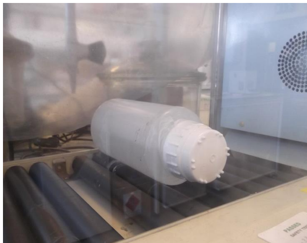
Figure 1.4: A typical low-profile roller and temperature controllable incubator system used in precipitation polymerisation reactions
