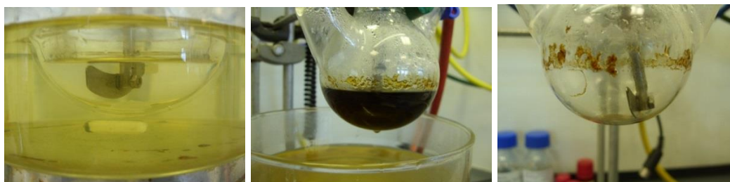
Figure 2.7: Photographs of KA41 after the addition of NaOH (left), at the end of the reaction (centre), and of the polymer stuck to the flask after the reaction mixture was removed (right)
