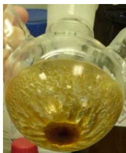
Figure 2.6: Photograph of the product obtained (sample KA29) from the reaction of poly(VP), formaldehyde solution, sodium hydroxide solution and ethanol
