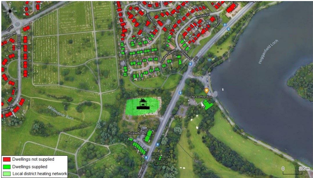
Figure A1.7. Local district heating network able to supply a nearby dwellings.
