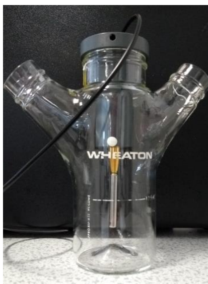
Figure 29: Needle hydrophone arrangement within the Celstir vessel, omitting the latex rubber sheath for clarity.
