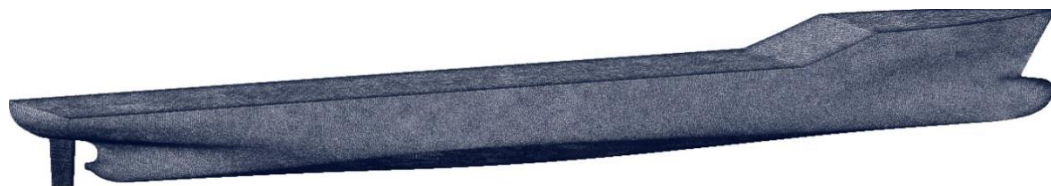
Figure 5.6 Surface mesh on the hull and rudder.
