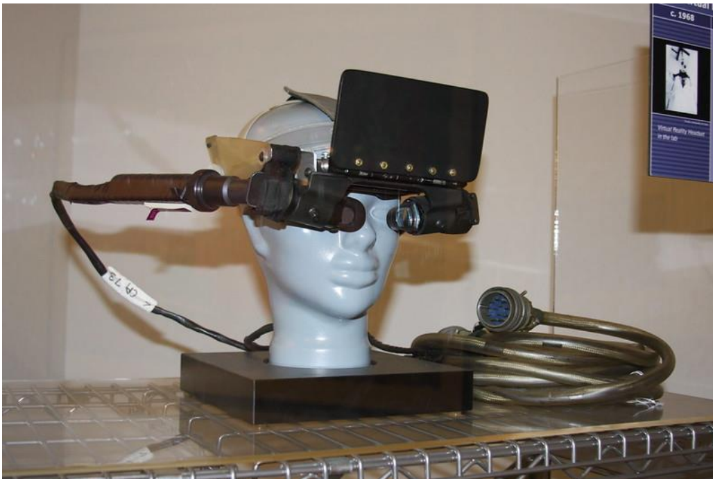
Figure 2.2 – Ivan Sutherland’s 1968 prototype headset ( photo used with permission from (Pargon, 2008), under CC BY 2.0 )
