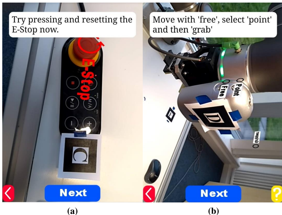
Figure 9.2 – Screenshots from the instructional app showing AR content overlaid onto (a) the robot stick, and (b) the Cobot arm
