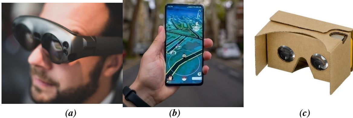
Figure 2.3 – Examples of current AR devices (a) Magic Leap AR headset (photo by Bram Van Oost, used with permission under Unsplash license), (b) AR app viewed on a smartphone phone (photo by Mika Baumeister used with permission under Unsplash license), and (c) a Google Cardboard AR viewing device
