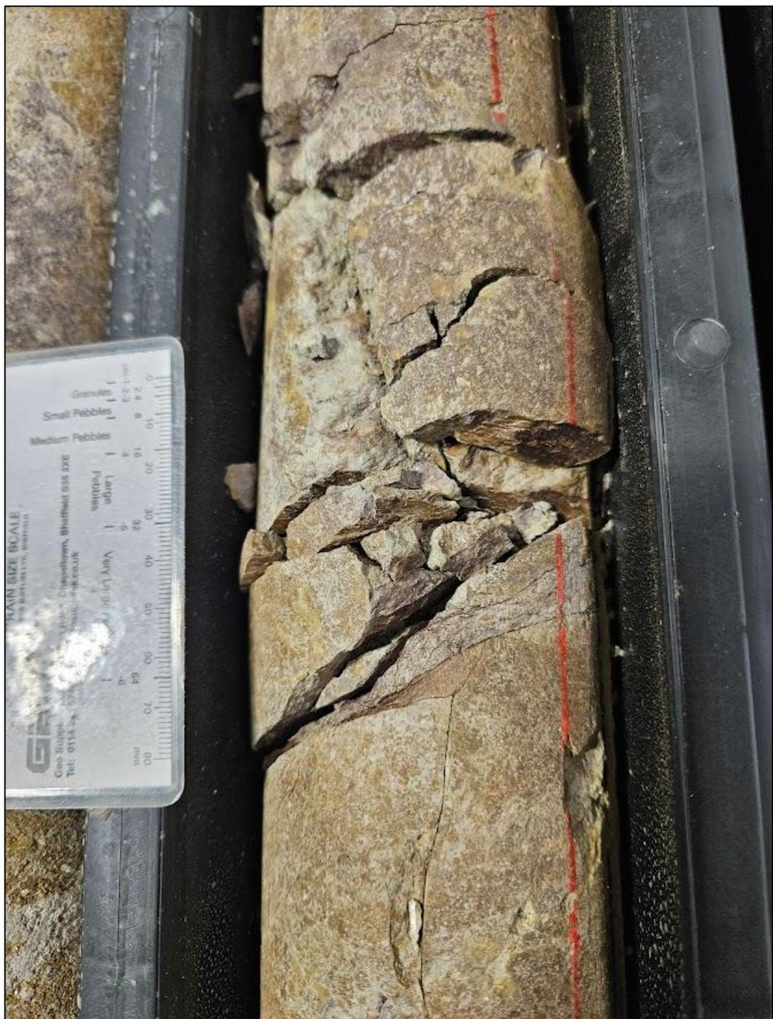
Figure 4-2 – Fractured palaeosol section in the Harvey-2 core. Multiple fracture orientations and angles, likely caused by a mix of drilling-induced fractures and the exploitation of existing sedimentary (pre-tectonic) structures by drilling.
