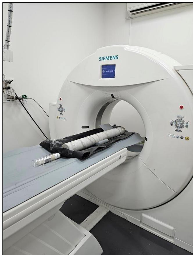
Figure 4-7– Siemens medical X-ray CT scanner SOMATOM Definition AS.
