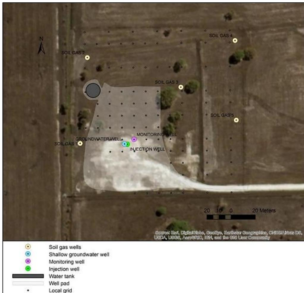
Figure 3-2 – Aerial view of the ISL showing the Harvey-2 (Injection well, green) and surrounding groundwater (blue), monitoring (purple) and soil gas wells (beige) (Myers et al., 2020).
