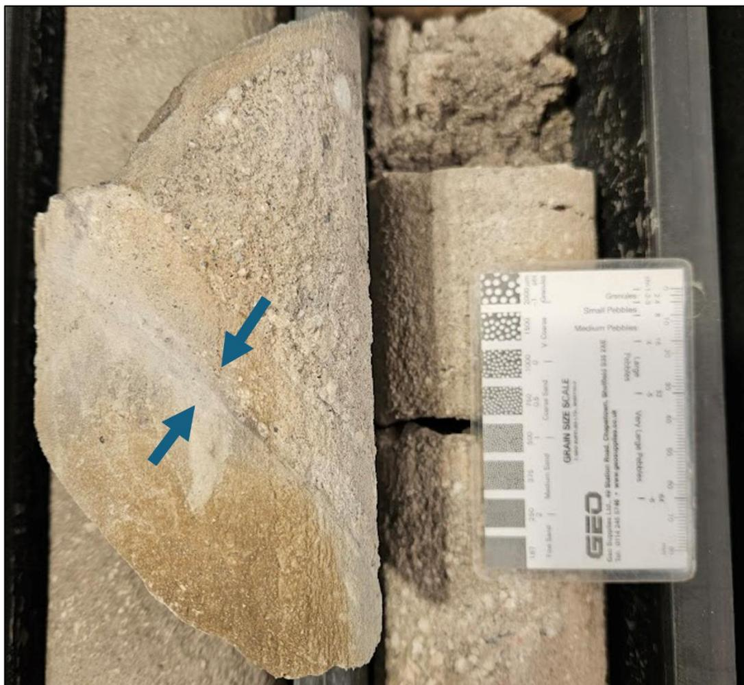
Figure 4-3 – Tectonic fracture in coarse sandstone from ~730m depth (Yalgorup Member) in the Harvey-2 core. Any displacement was not able to be estimated, as no markers are offset.
