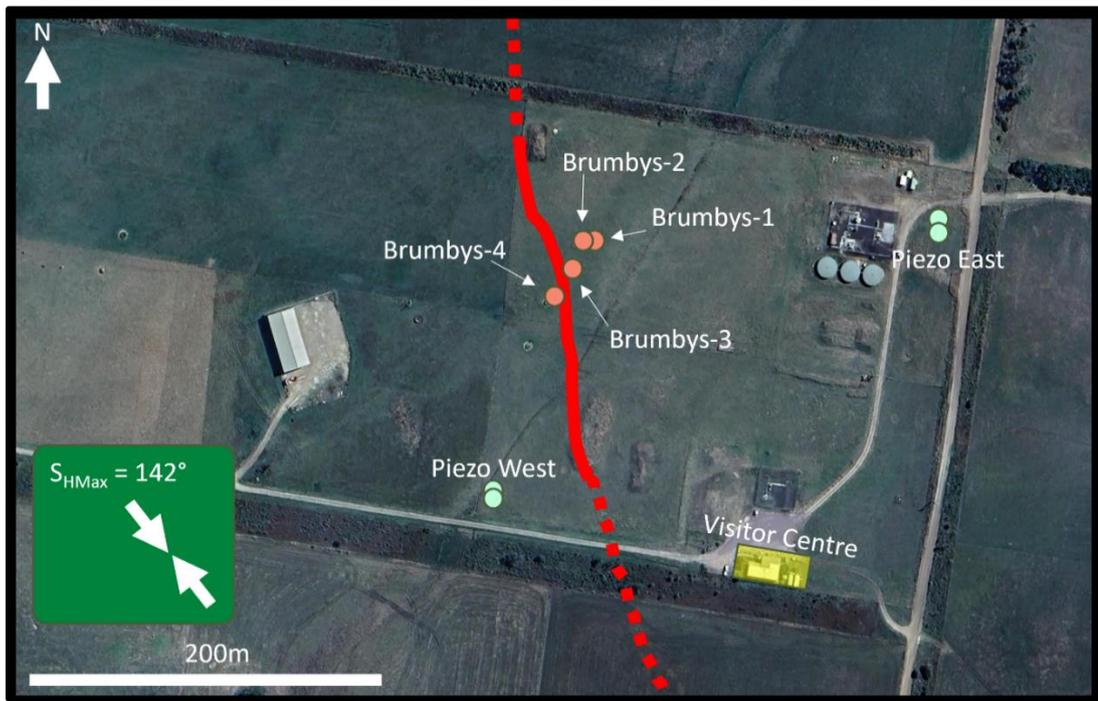
Figure 3-21 – Map showing the layout of the Otway International Test Centre (OITC), including Brumbys wells (orange) and monitoring wells (light green). Red line depicts the surface trace of the Brumbys Fault (solid = 3D seismic trace, dashed = regional 2D seismic). Satellite image from Google Maps ©2024 Airbus, CNES/Airbus Maxar technologies, Map Data ©2024.
