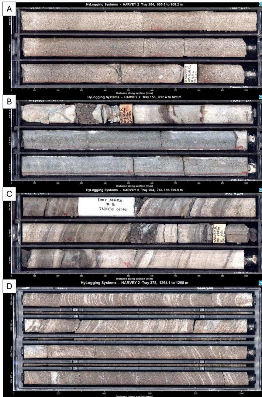
Figure 5-1– Examples of the variability of the undeformed sandstone in the Harvey-2 core. A: Tray 254 (Start depth = 905.5m, Yalgorup Member) – typical coarse-grained sandstone, some grit. B: Tray 150 (Start depth = 617.4m, Yalgorup Member) - Green coloured sandstone. C: Tray 204 (Start depth = 766.7, Yalgorup Member) – Interbedded sandstone, mudstones and palaeosols. D: Tray 378 (Start depth = 1264.1m) – Cross-bedded sandstone of the Wonnerup member.
