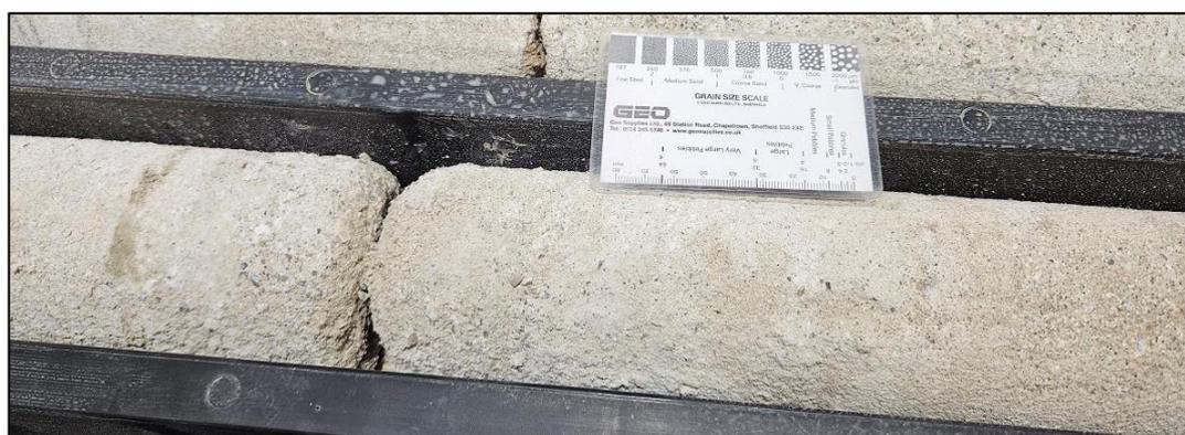
Figure 4-1 – Drilling induced fracture at ~790m depth (Yalgorup Member) in sandstone in the Harvey-2 core.
