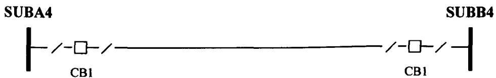
Figure 2-6 Single line diagram representation of a 400kV feeder circuit
