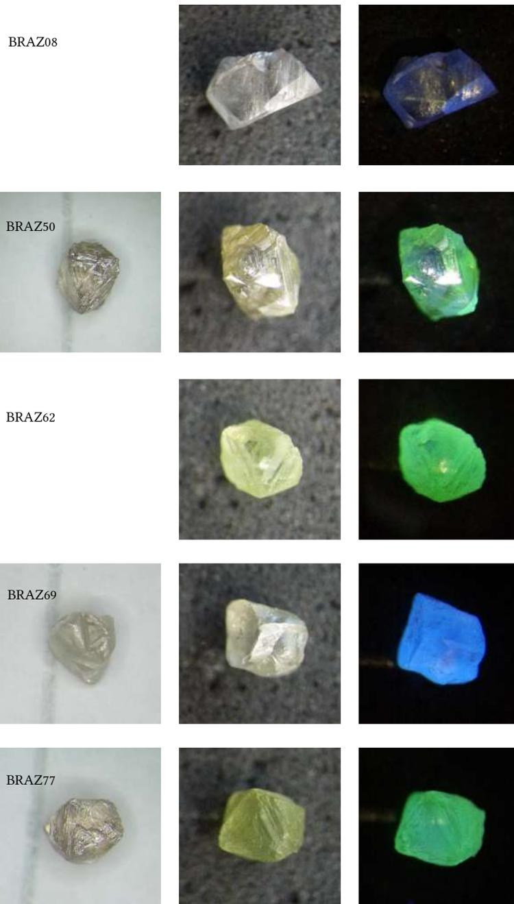
Figure 5.23: Natural diamond samples before and after HPHT treatment
