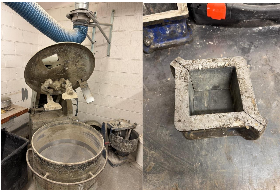
Figure 9: The laboratory mixing machine and model cubes (author's own photo).
