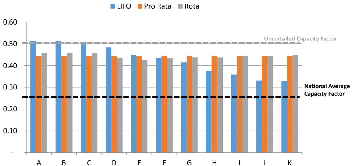
**Figure 5-13 Average annual capacity factor for generators on a network with a single GSP constraint**
