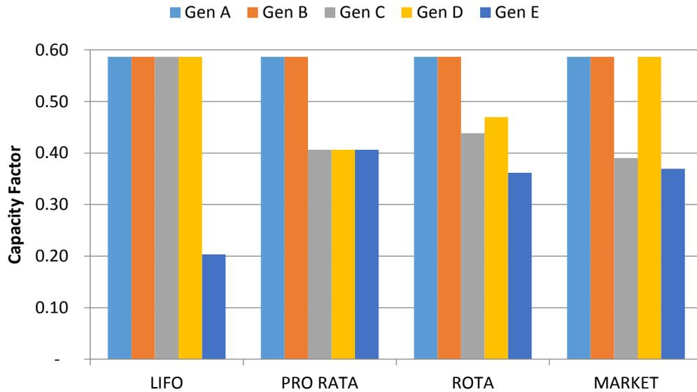
**Figure 4-19 Study B Results: Impact of CF on non-firm wind generators in a six bus network with a local constraint**
