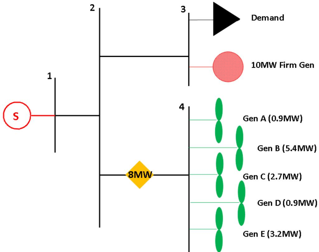
Figure 4-11 Study A: Network diagram
