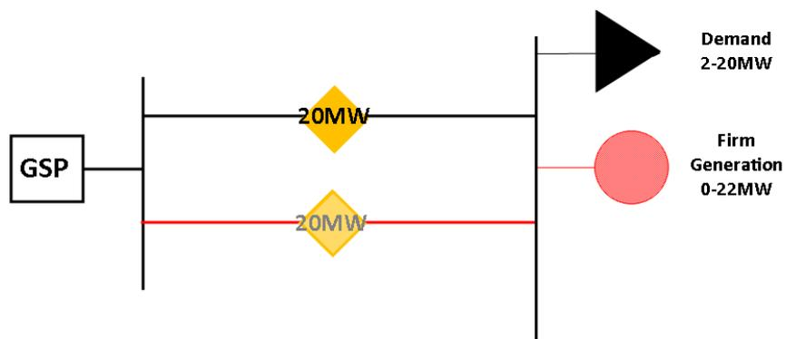
**Figure 1-2 Schematic showing firm network capacity under N-1 conditions**
