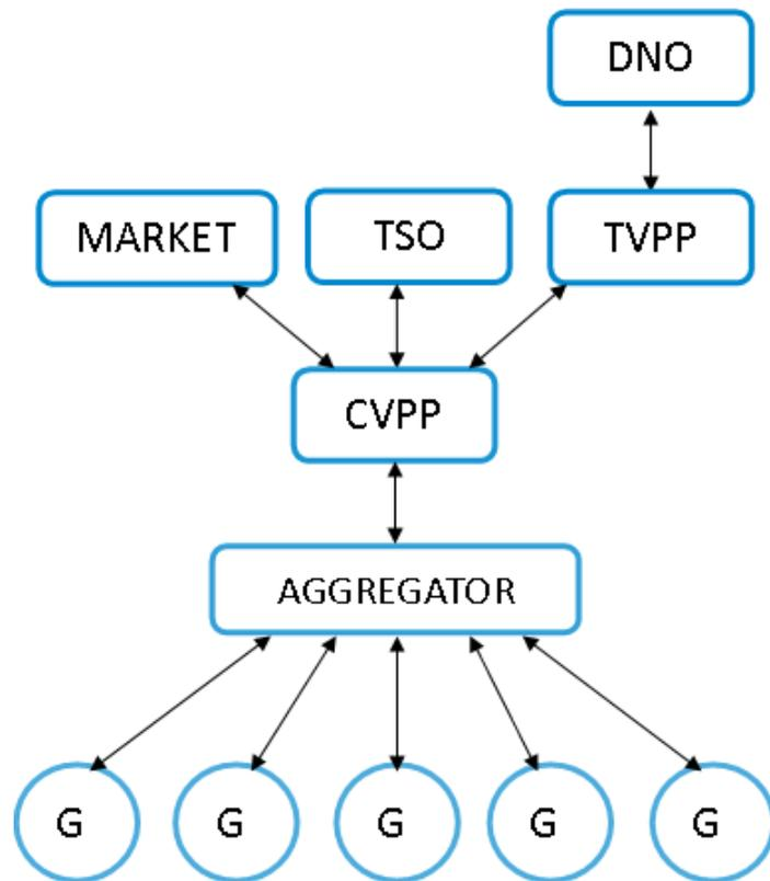
Figure 2-20 Diagram illustrating the operation of a VPP
