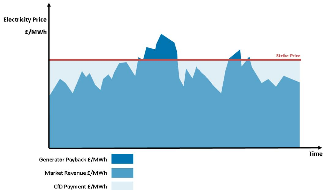
**Figure 2-4 Diagram of how contracts for difference will operate**
