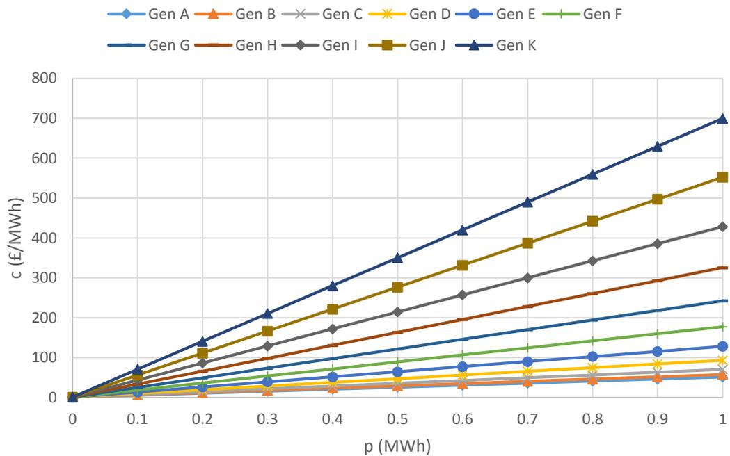
**Figure 4-1 Graph showing cost functions used to apply a LIFO arrangement. The generator with the highest cost gradient will be curtailed first**
