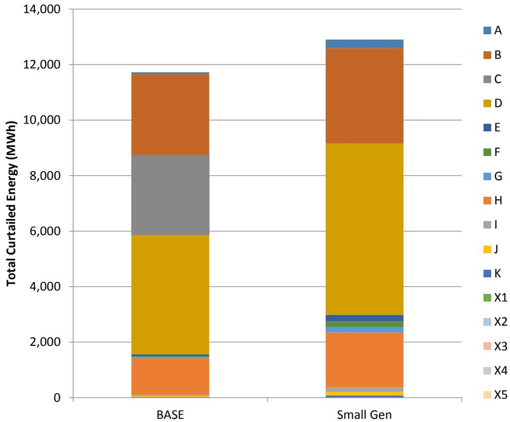
**Figure 5-45 Total curtailed energy for the small generator scenario compared with the base case market arrangement**
