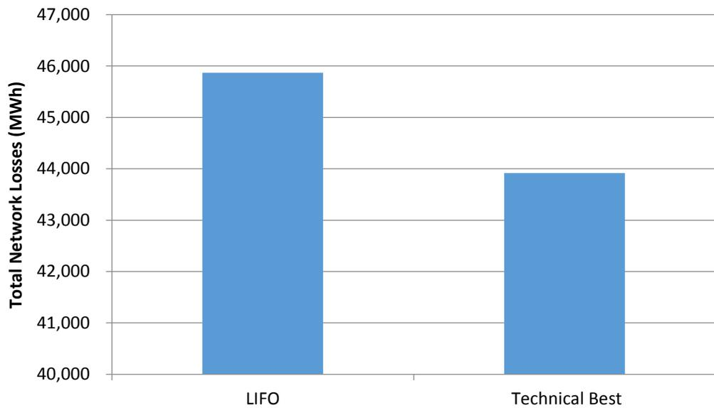
**Figure 5-17 Comparison of the losses experience on the network under a LIFO arrangement and a 'Technical Best' arrangement which is designed to minimise losses**
