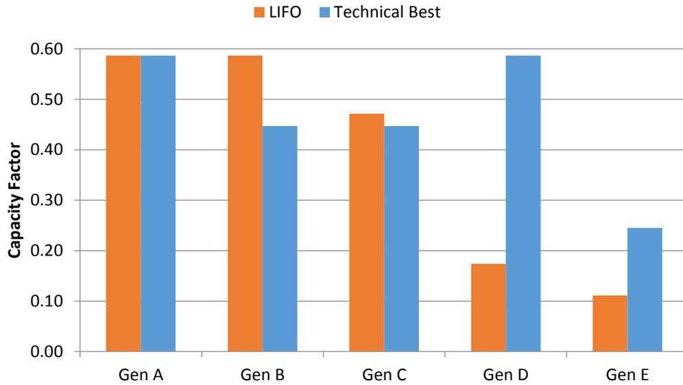
**Figure 4-27 Study C Results: Capacity factor of non-firm generators under a ‘technical best’ arrangement compared with the LIFO capacity factors**
