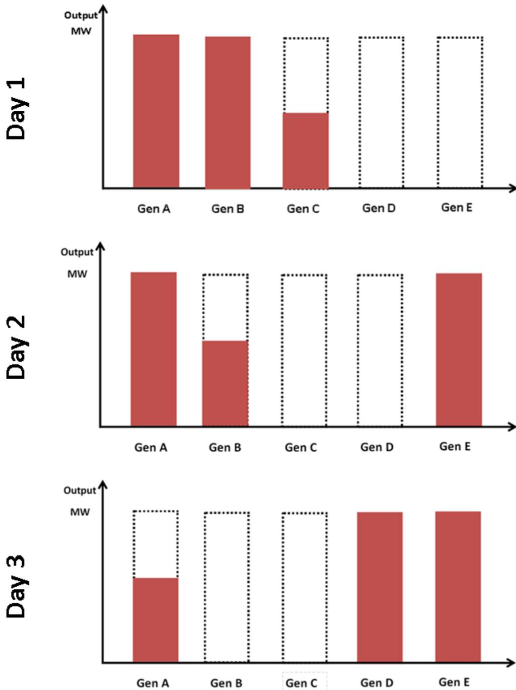
Figure 4-3 Diagram of how curtailment is applied during a Rota arrangement
