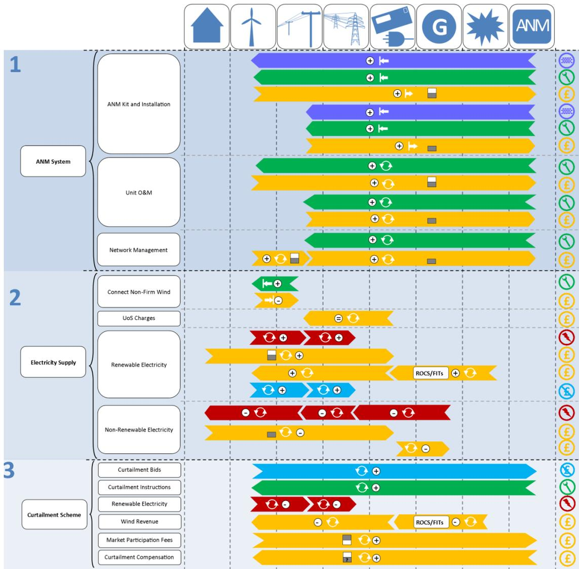
**Figure 6-10 Business model of ANM scheme operating a Market PoA (Based on models developed by ECI [12])**
