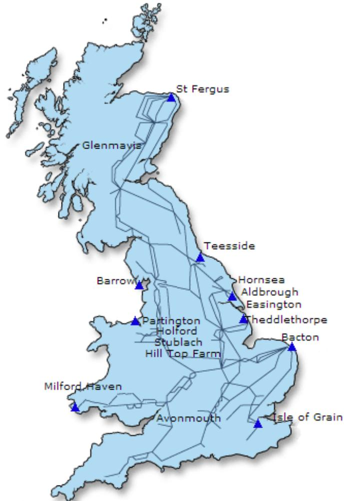
**Figure 2-9 GB gas transmission system with entry terminals shown [69]**
