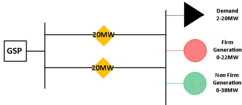
**Figure 1-3 Schematic showing firm and non-firm capacity by utilising ANM control systems**
