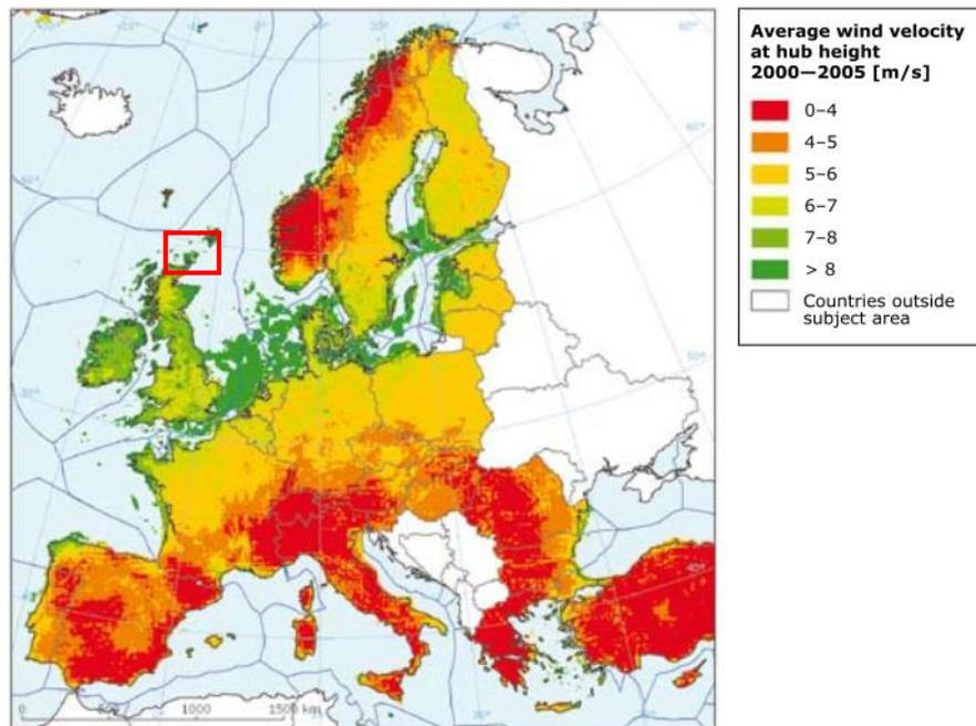
**Figure 5-1 Wind resource map of Europe, showing that the UK has a high resource, and in particular the Orkney Islands (highlighted by the red box) off the north coast have a very high wind resource [166]**
