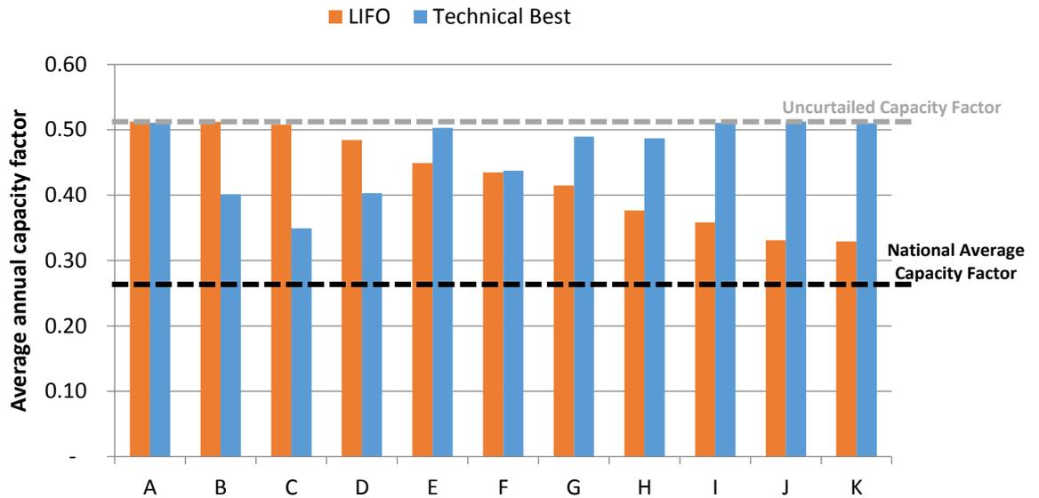
**Figure 5-18 Average annual capacity factor for non-firm generators subjected to a 'technical best' curtailment strategy and compared with the original LIFO arrangement**
