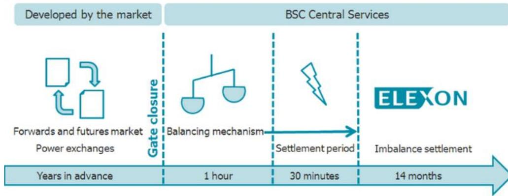
**Figure 2-3 Overview of the settlement and balancing process [18]**
