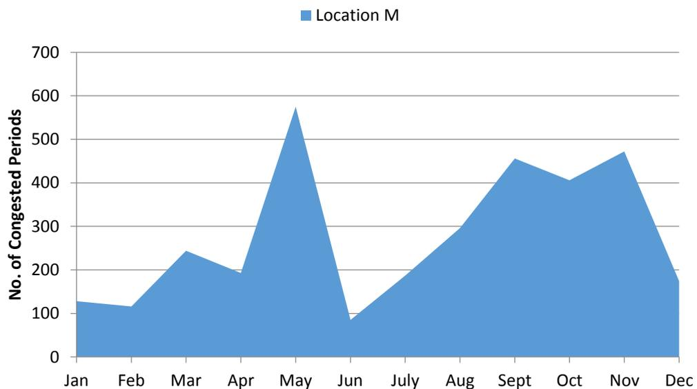
**Figure 5-10 Number of constrained periods occurring during one year on the case study network. Each constraint period represents a 30 minute time step**
