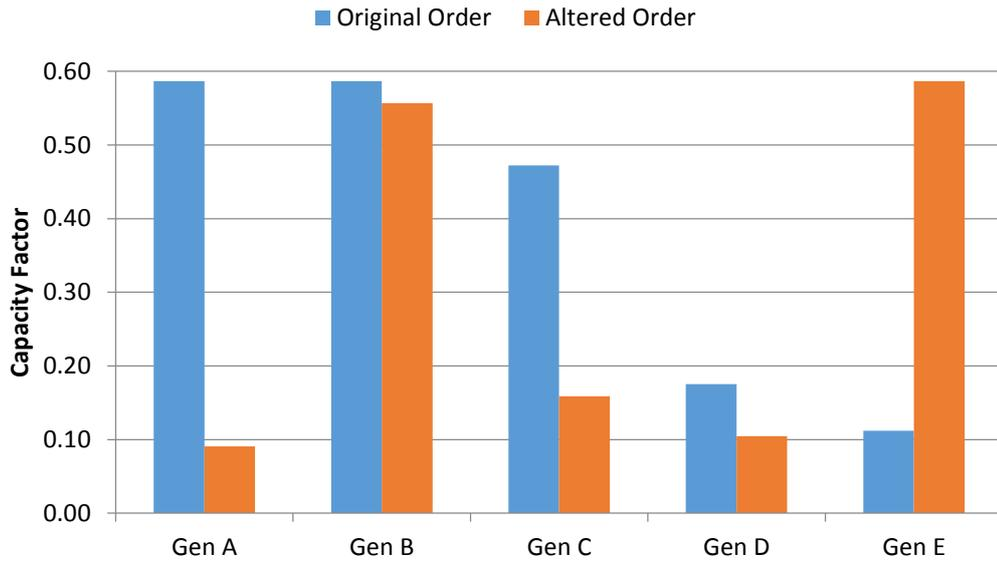
**Figure 4-16 Graph showing the impact on capacity factor when the priority stack order is changed. Generator A and Generator E have had their positions switched in the second series.**
