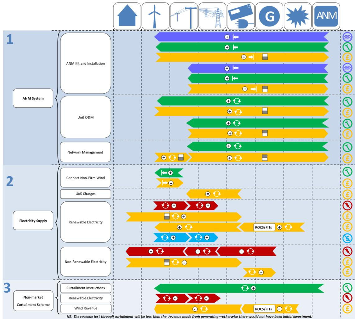
**Figure 6-8 Business model of ANM Scheme operating non-market PoA (Based on models developed by SuperGen HiDEF Distributed Energy Modelling project [12])**
