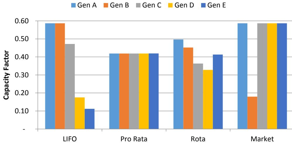
**Figure 4-13: Study A Results: Impact of capacity factor on non-firm wind generators in a four bus network with a single constraint**
