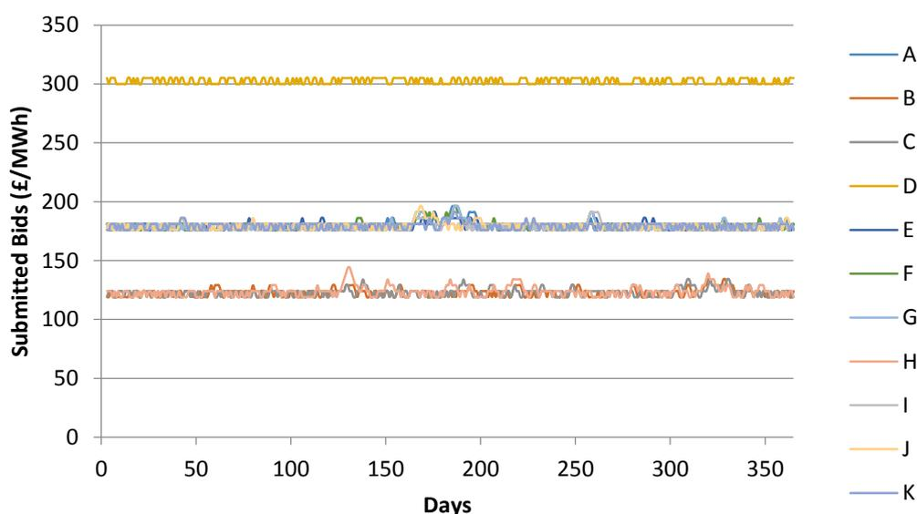
**Figure 5-38 Bid behaviour in a market arrangement when one generator bids at a high price level**
