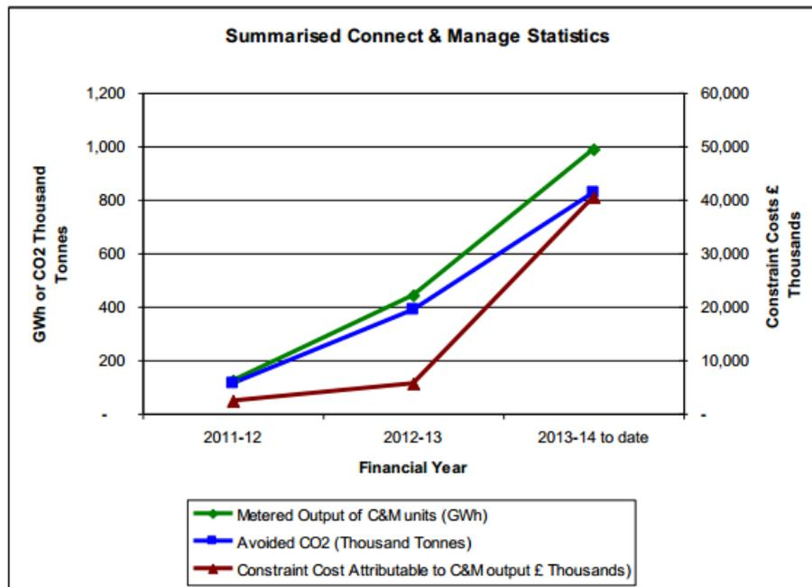
**Figure 2-5 Summarised Connect and Manage statistics demonstrating the increase in connected generation since 2011 in GB [51]**
