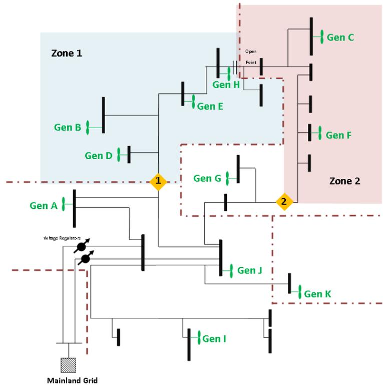
**Figure 5-4 Location of local constraints and Pro Rata curtailment zones.**
