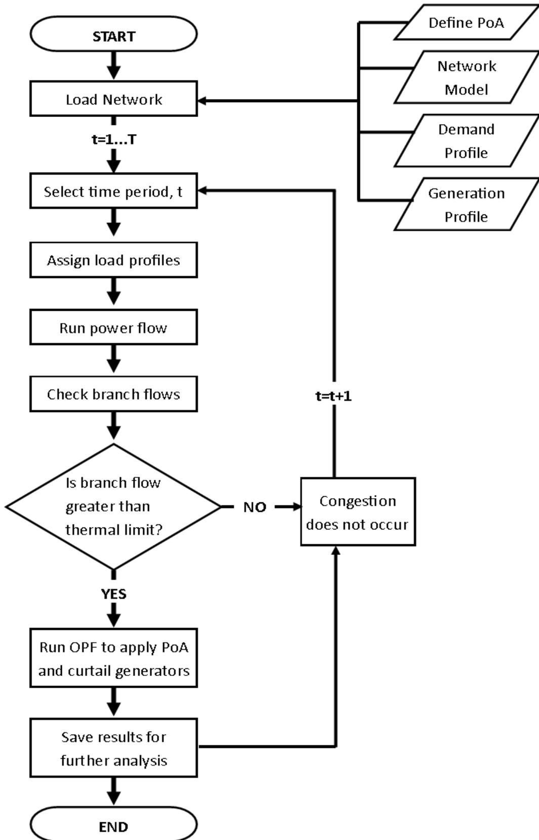
Figure 4-8 Annual Constraint Analysis Modelling Process
