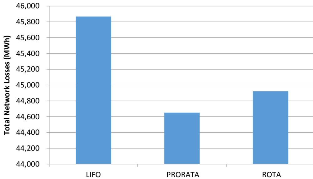
Figure 5-12 Diagram of losses on a network with a single constraint at GSP under different arrangements
