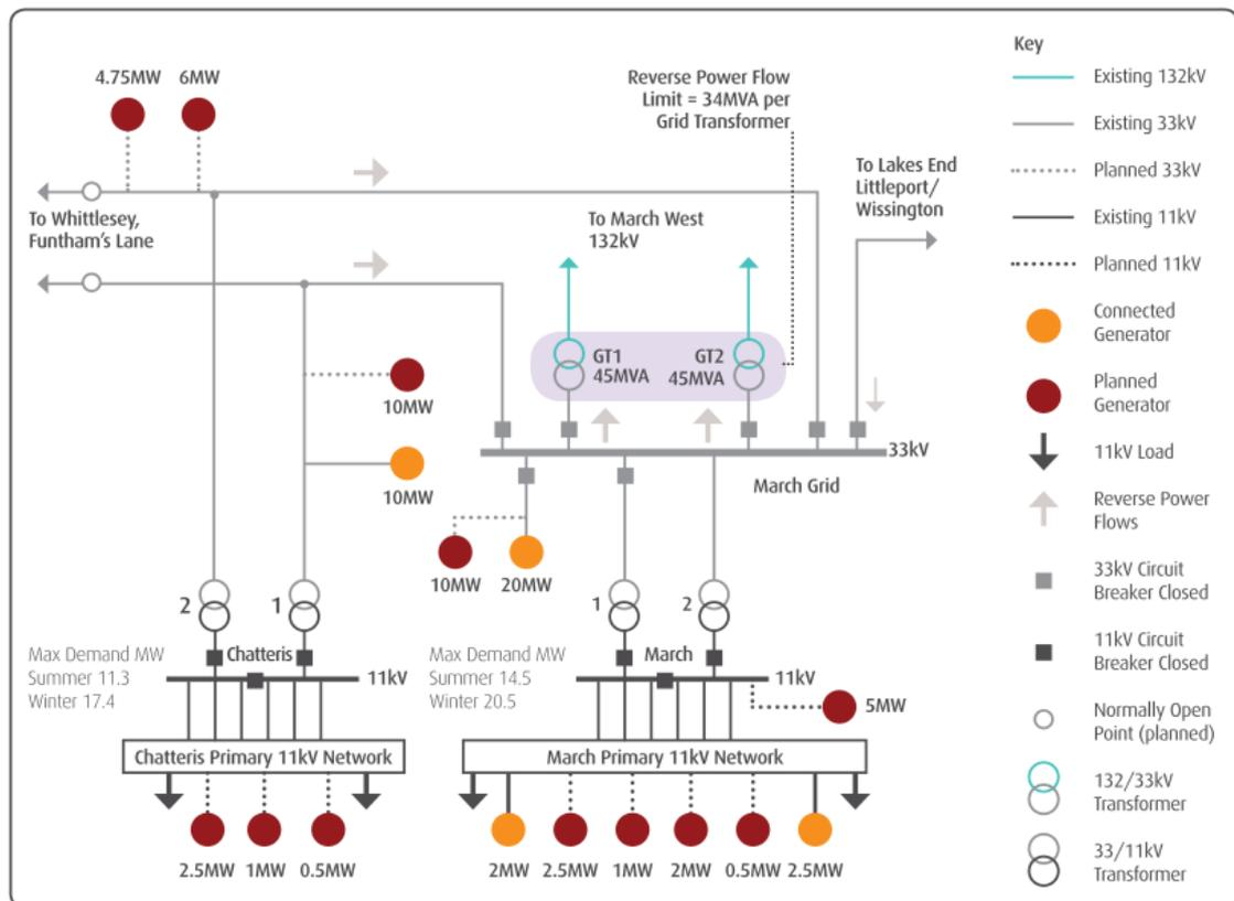
Figure 2-16 Simplified diagram of March grid [10]
