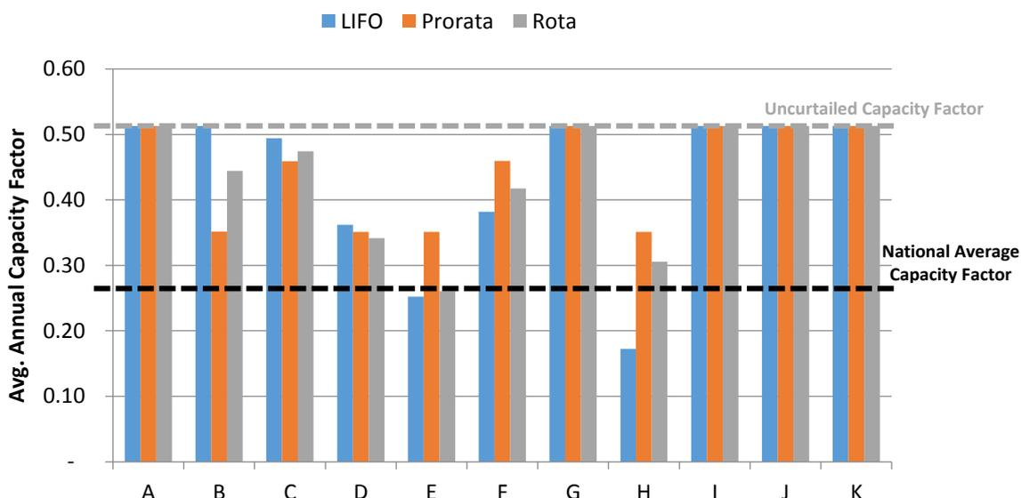
**Figure 5-8 Average Annual Capacity Factor for generators on a network with local constraints**
