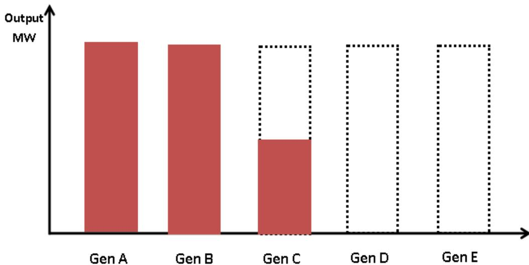
**Figure 4-2 Diagram of how curtailment is applied during a LIFO arrangement**
