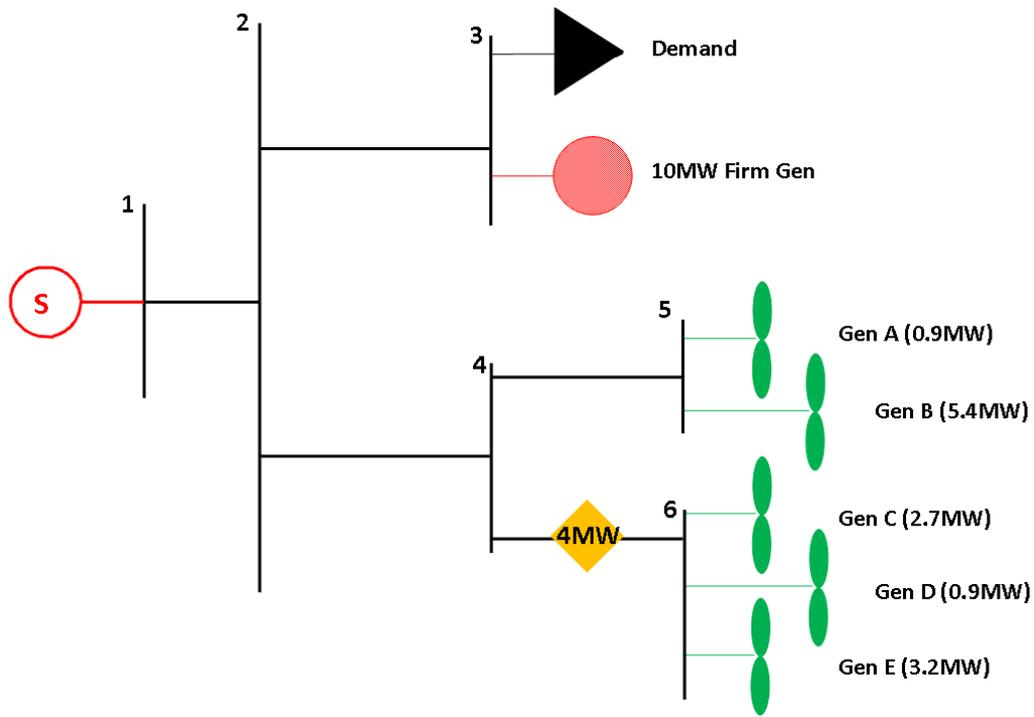
**Figure 4-17 Five bus example with local constraints**
