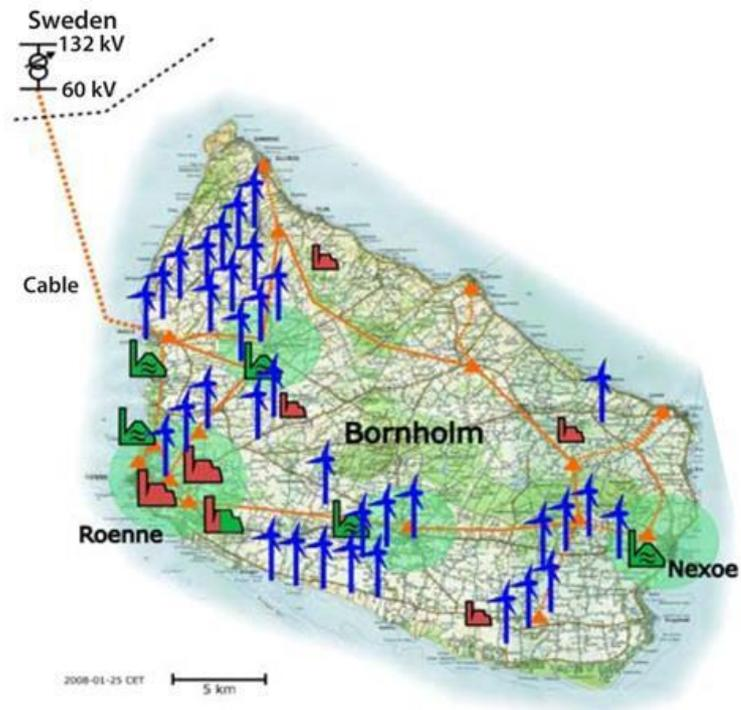
**Figure 2-21 Diagram of Bornholm Smart Grid project [101]**
