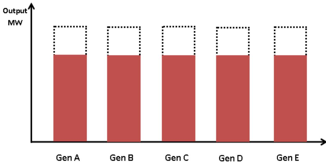
Figure 4-4 Diagram of how curtailment is applied during a Pro Rata arrangement
