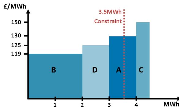
Figure 4-7 Diagram of generator curtailment
