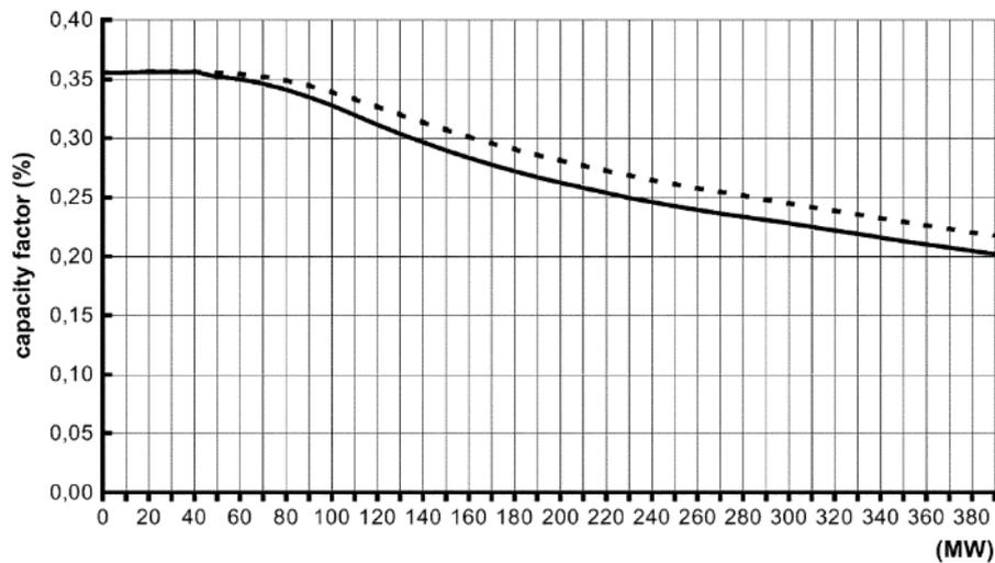
**Figure 2-7 Estimated variation of capacity factor versus total wind capacity. The solid line indicates typical operation; the dash line is the result using preventative control [66]**
