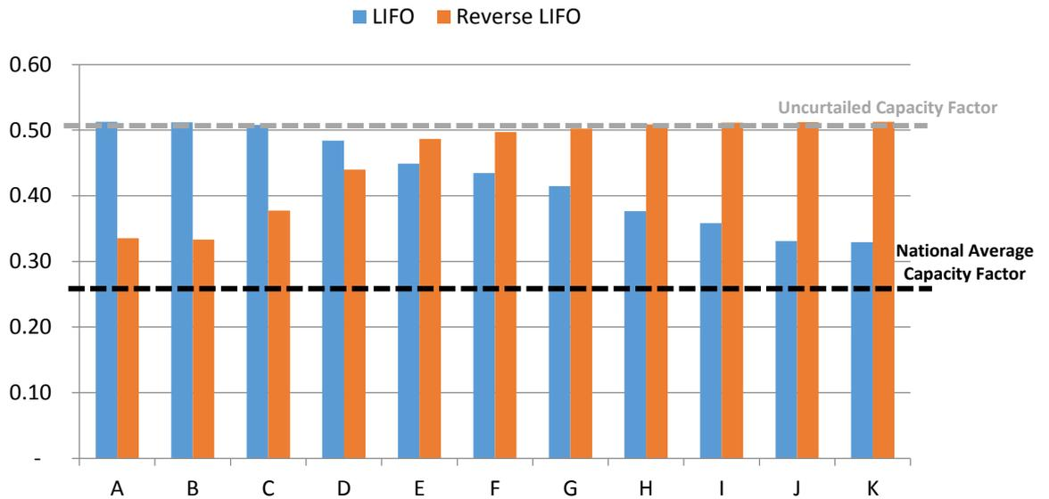
**Figure 5-16 The average annual capacity factors for a LIFO arrangement, and a second LIFO arrangement where the curtailment order has been reversed**
