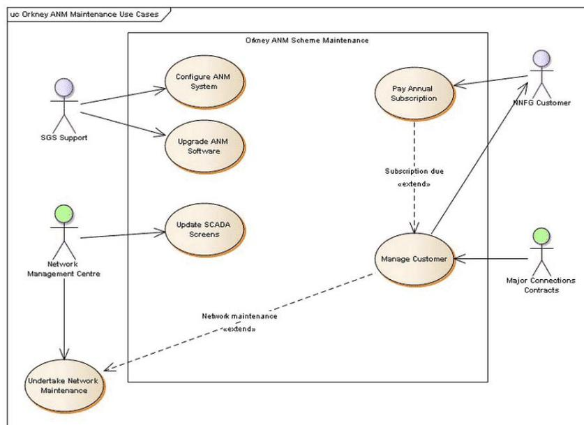
**Figure 6-6 SSEPD diagram explaining Orkney ANM maintenance use cases [186]**
