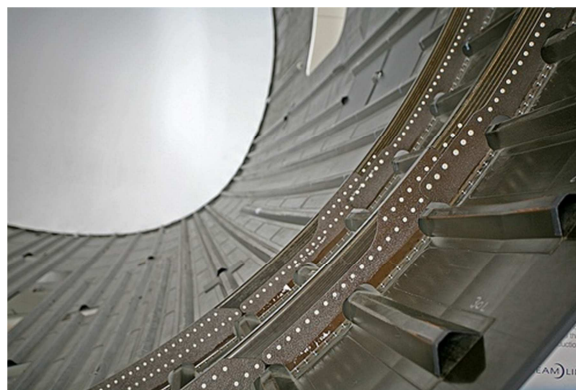
Figure 2.1 – A disassembled carbon fibre fuselage section of the Boeing Dreamliner 787 in Everett, Washington (Source: Wikipedia)
