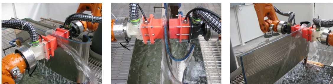
Figure 7.13 – Through-transmission scan of a wing leading edge sample.
