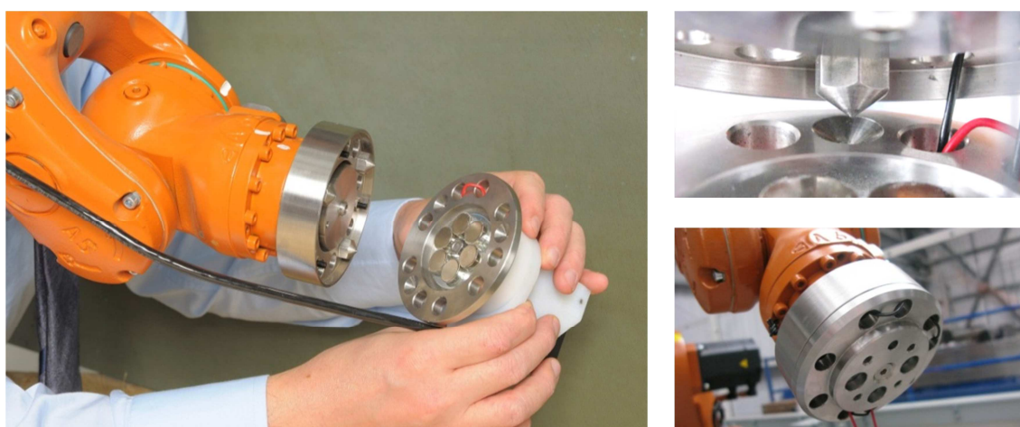
Figure 6.8 – Magnetic holder mounted to the KUKA KR16 L-6 robot extremity.
