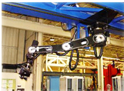
Figure 2.9 – AUSS 6-axis robot suspended on sliding gantry.
