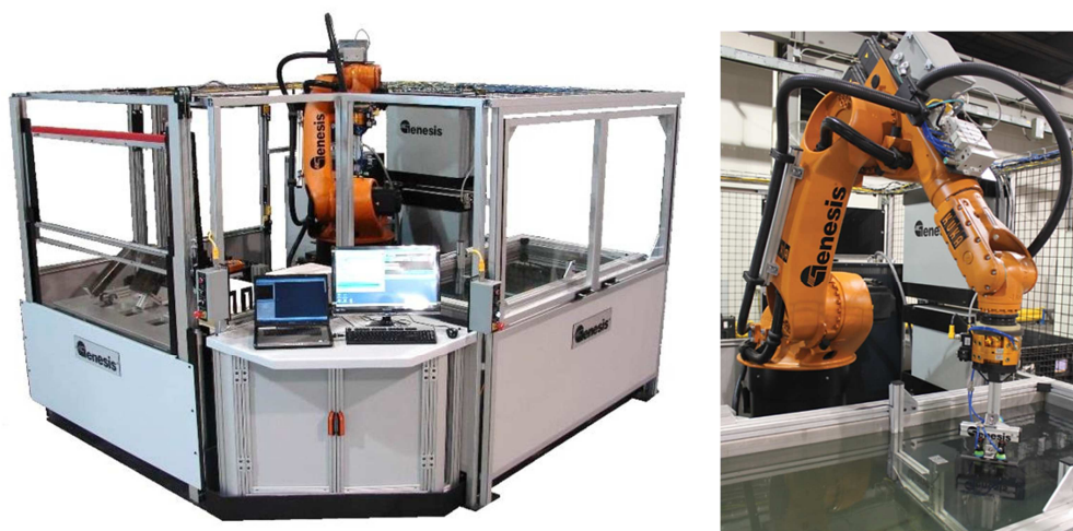
Figure 2.13 – NDTS & Genesis NSpect210 system.
