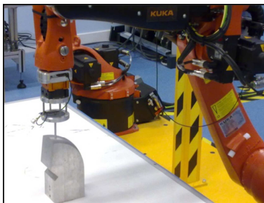
Figure 3.23 – Robotic arm at the beginning of the raster scan.
