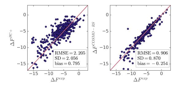
FIGURE 7.9: Computed solvation free energies of a number of compounds in polar solvents (as defined in table 7.4) against experimental data. COSMO-RS results are taken from Ref. 219. All values are in kcal/mol.
