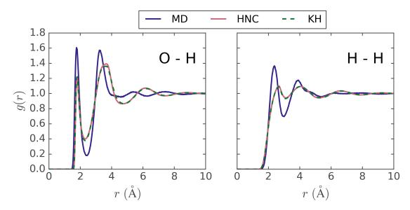
FIGURE B.1: Site-site radial distribution functions of SPC/E water (cSPC/E in case of DRISM calculations).
