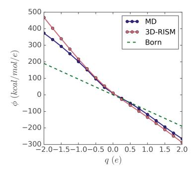
FIGURE 5.5: Electrostatic potential inside the soft solute with  $\sigma = 3.8 \,\text{Å}$  and  $\epsilon = 0.125 \,\text{kcal/mol}$  depending on its charge.
