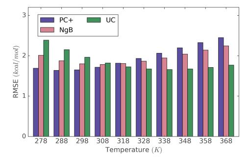
FIGURE B.4: Root mean square error of solvation free energy of 3D-RISM models on the Chamberlin dataset. Unlike figure 6.6, here we do not vary temperature in 3D-RISM calculations, using the value of  $\Delta G$  at 298 K for all comparisons.
