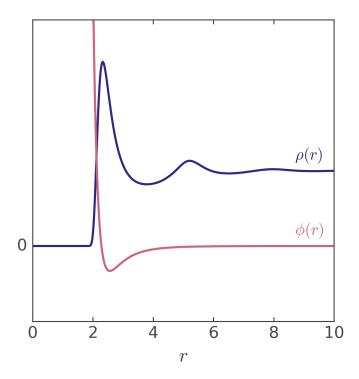
FIGURE 1.2: A particle with a spherically symmetric potential  $\phi(r)$  is placed at the origin. The surrounding solvent rearranges, forming multiple solvation shells. The dependence of its average density  $\rho(r)$  can be obtained using classical density functional theories. The units are arbitrary.
