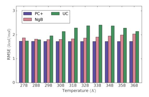
FIGURE 6.6: Root mean square error of solvation free energy of 3D-RISM models on Chamberlin dataset depending on temperature.
