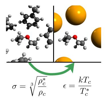
Figure 7.5: The basic idea behind coarse graining used for 3D-RISM calculations. The real liquids are approximated as spheres interacting via Lennard-Jones potentials with parameters deduced using equations shown on the figure above.
