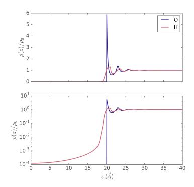
FIGURE 4.7: Distribution of water oxygens (blue) and hydrogens (red) in a large box with  $u_O = \infty$  for z < 20 Å. You can see that some hydrogens can be found arbitrarily far away from the oxygens.
