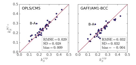
FIGURE 7.3: Setschenow's constants by 3D-RISM/PC+ with Dang salt model compared to experimental measurements by Endo et al. Results on the left and right figures are obtained with OPLS/CM5 and GAFF/AM1-BCC force fields respectively. B-A stands for bisphenol A. The values are in l/mol.
