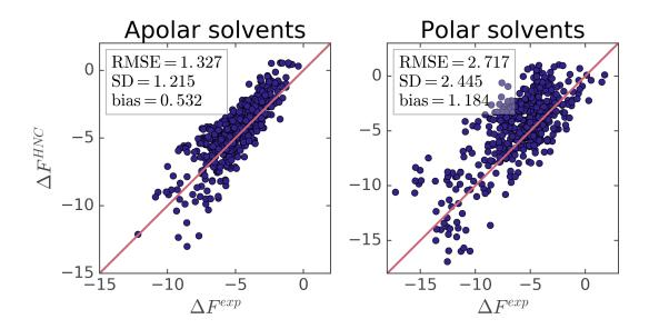
Figure B.5: Comparison of computed (3D-RISM/HNC) and experimental solvation free energies in polar and apolar solvents (as defined in section 7.5). All values are in kcal/mol.
