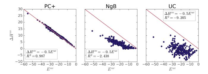
FIGURE 6.7: Correlations between solute-solvent and solvent reorganization energies.  $\mathbb{R}^2$  stands for coefficient of determination. All values are in kcal/mol.
