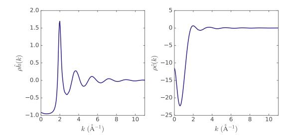
FIGURE 3.3: Fourier transforms of the total correlation function (left) and the direct correlation function (right) from figure 3.2.
