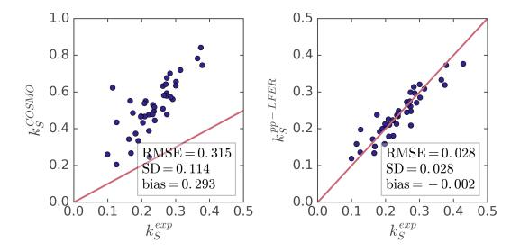
FIGURE 7.2: Accuracies of Setschenow's constants predictions by COSMO-RS (left) and pp-LFER model (right). Both experimental and computed values are taken from Ref. 178. All values are in l mol<sup>-1</sup>.
