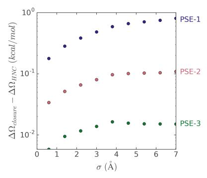
FIGURE 4.8: Solvation free energies of Lennard-Jones solutes with  $\sigma$  given on x axis and  $\epsilon = 4 \, \text{kcal/mol}$ . On y axis you can see the difference in free energies by PSE-n and HNC closures.
