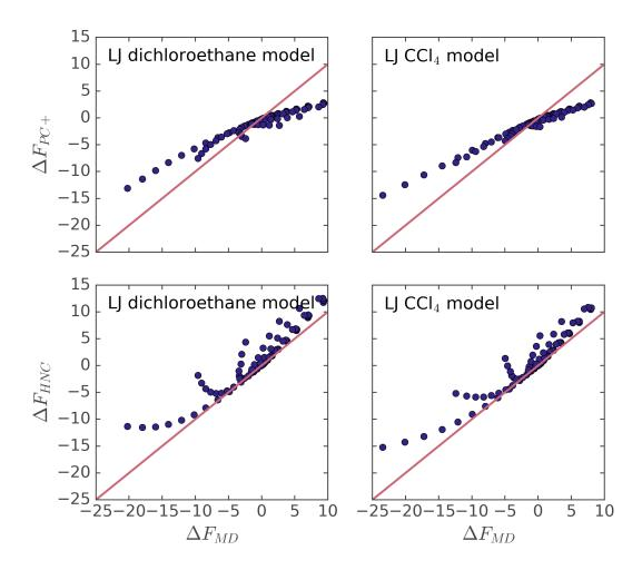
FIGURE 7.7: Calculated Lennard-Jones solutes solvation free energies against MD data. Dichloroethane and CCl<sub>4</sub> models are defined in table 7.3. All values are in kcal/mol.
