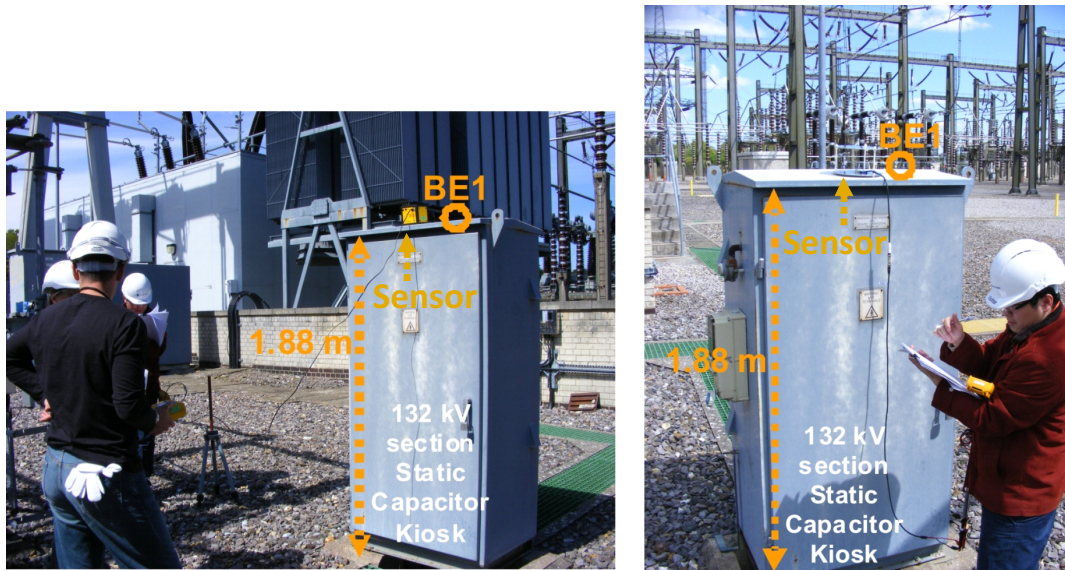
Figure 3.10: Left - Narda EFA-300 field analyser set, Right - Circular field sensor. Both sets of instruments were used to measure the field strength at BE1 (please refer to Table 3.2 for the precise location).
