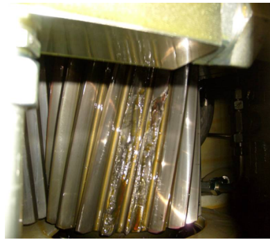
Figure 5.3: Broken pinion on intermediate shaft
