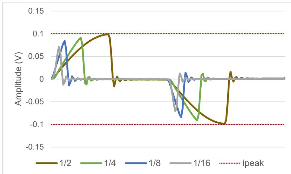
Figure 5.29: ADC “leading” sampled waveforms.
