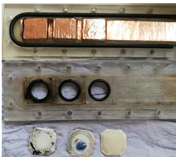
Figure 72: Photograph of a sample holder for anodizing with a copper tape for connecting Al samples.
