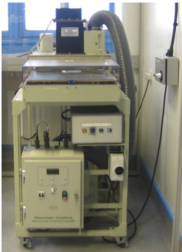
**Figure 4.1. Sherman Treaters GX10 corona treatment machine used in the high power corona treatment of substrates.**
