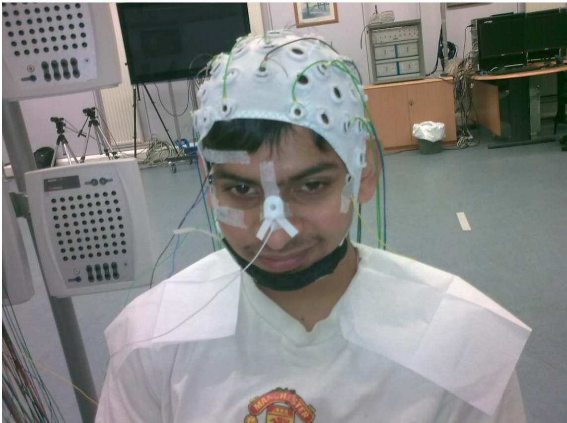
Figure 3.2: Pilot subject with the electrode cap, the nose reference and vertical and horizontal electrodes which were used to capture the artefact due to movement of eyes.
