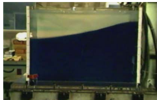
Fig 7.5 Evolution of fluid during sloshing at time = 1.175s
