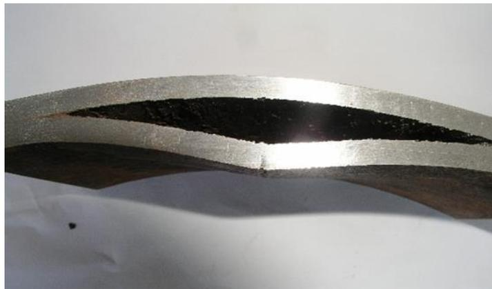
**Figure 3.10 Example of Hydrogen Induced Cracking (King Fahd University of Petroleum & Minerals, 2018)**
