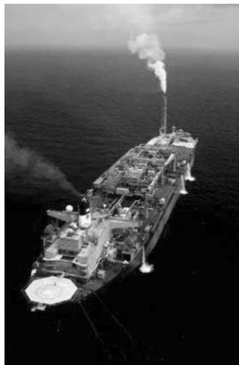
**Figure 2.9 Floating Production, Storage and Offloading Vessel (Devold, 2013)**
