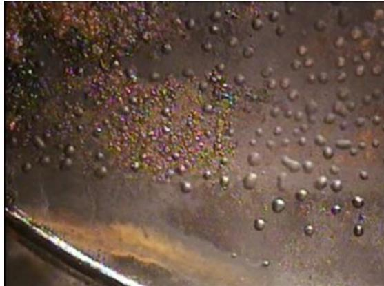
**Figure 3.9 Example of Hydrogen Blistering (Maverick Inspection Ltd, 2018)**
