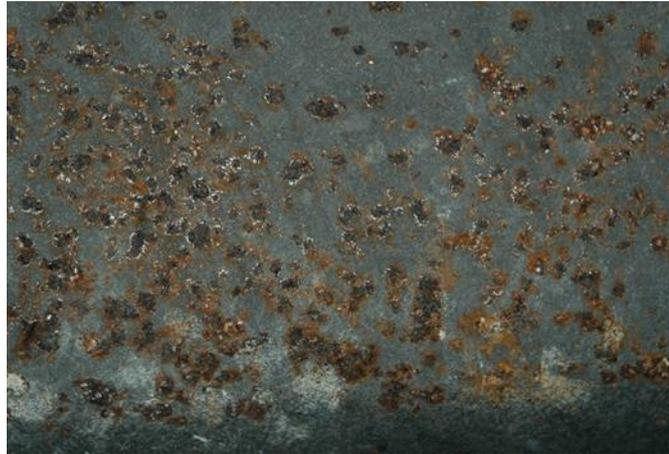
**Figure 3.5 Example of Pitting Corrosion of Steel (Steel Fabrication Services, 2018b)**
