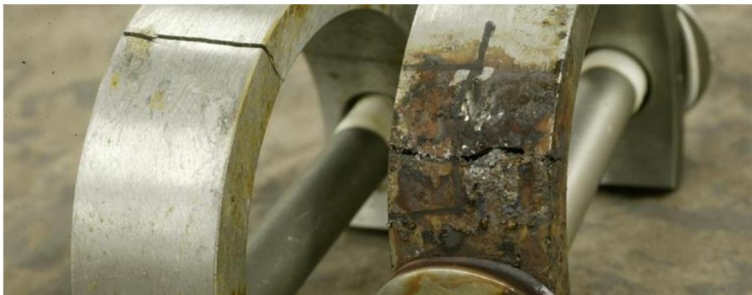
**Figure 3.8 Example of Stress Corrosion Cracking (Southwest Research Institute, 2018)**
