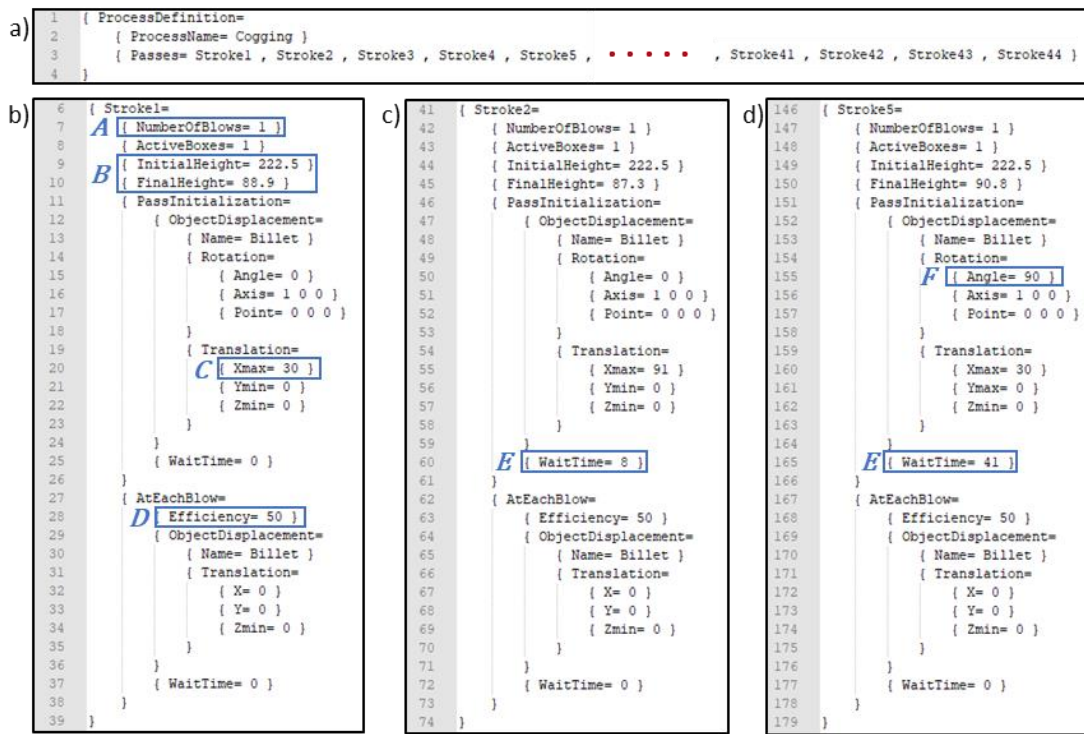
Figure 3.41 : Annotated screenshots of the *.mpfx file used in FORGE® for modelling the kinematic of both the screw press and the 316L grade ingot during C1 cogging; a) header section, and b) to c) the parameter sections for the 1 st , 2 nd and 5 th hits from the press, respectively. Note that this *.mpfx kinematic file describe 44 individual hits from the press, along 1545 lines.
