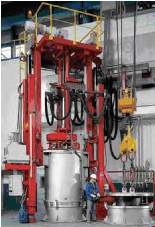
Figure 2.9 : Photograph of a 30-tonnes capacity vacuum arc remelting (VAR) furnace, (Reardon, 2011).
