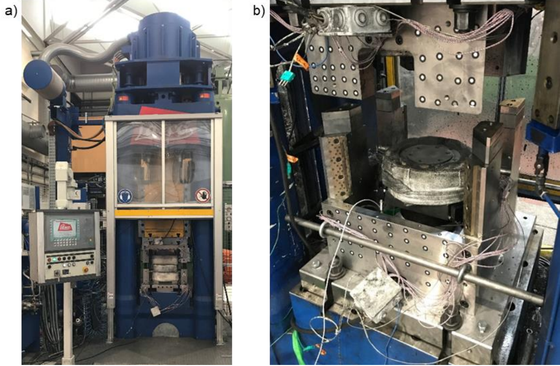
Figure 3.15 : a) The Lasco® SPR 400 screw press ( 28.9 \text{ kJ} at 680 \text{ mm.s}^{-1} ), and b) the associated tooling sets used for the upsetting tests conducted using this press.
