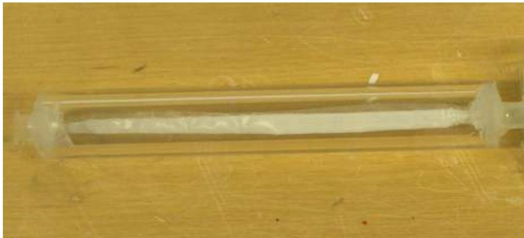
**Figure 4.4 – Celgard 2500 tube positioned within test housing, held in place with silicone rubber adhesive.**
