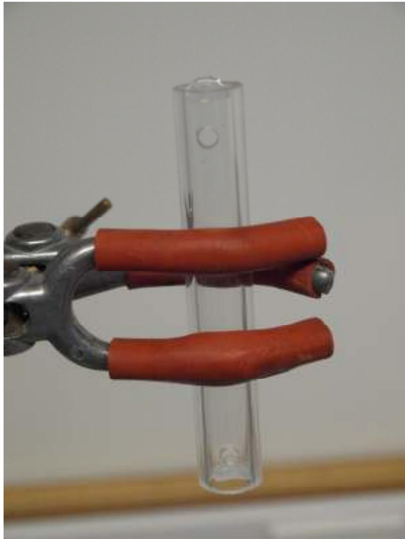
**Figure 4.2 – A completed test housing unit, with inlet and outlet holes visible.**
