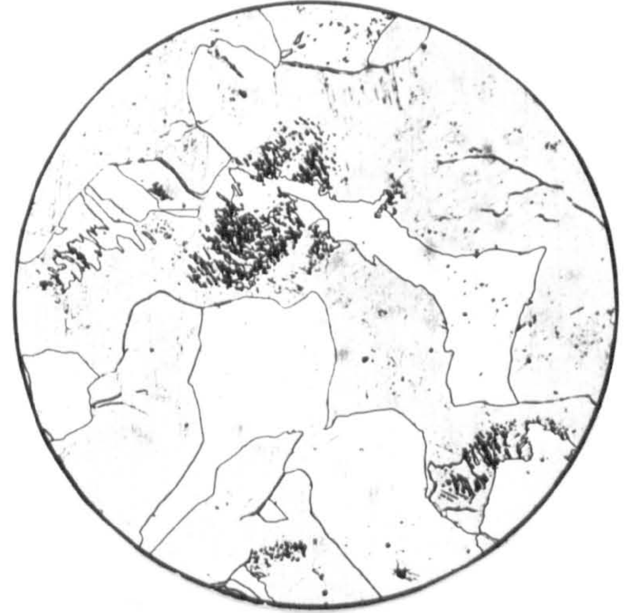
COOLING AT 0.17 s -1 FROM 1425 K
