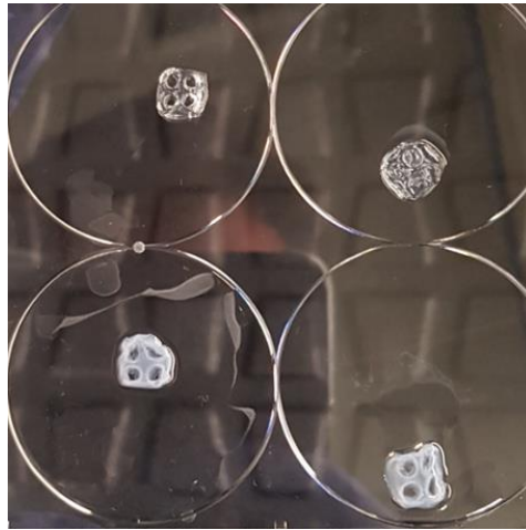
Figure 7.9: The 4 different types of patches after releasing them from the mould, but before placing them in medium. Top: alginate patches without (Left) or with 10 ng/ml VEGF (right). Bottom: Collagen patches without (left) or with 10 ng/ml VEGF (right)
