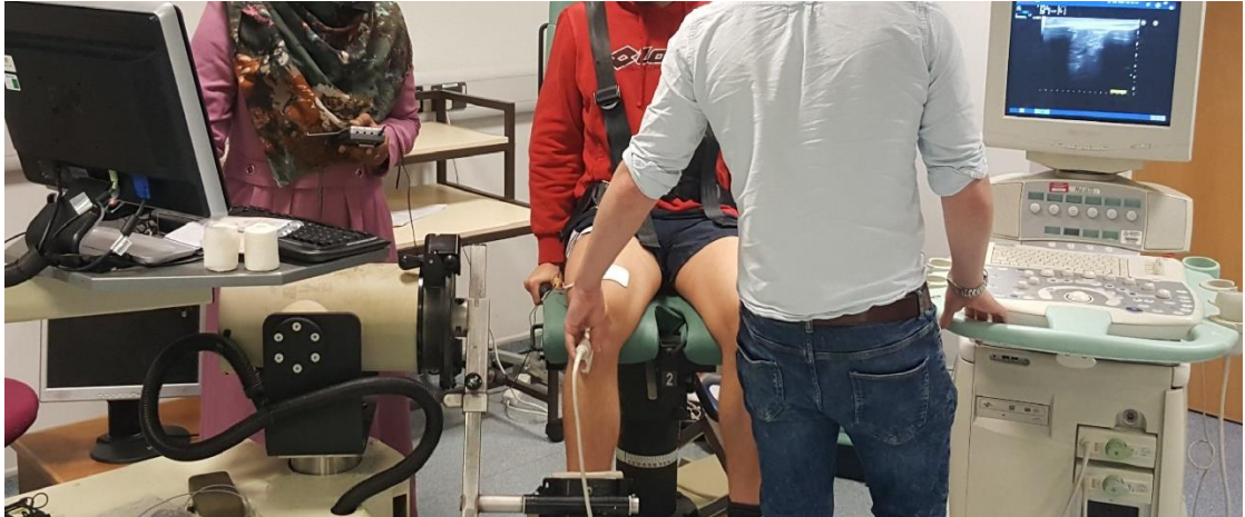
Figure 4.2: Measuring patellar tendon elongation using ultrasound probe placed on participant knee during electrical stimulation of thigh muscles
