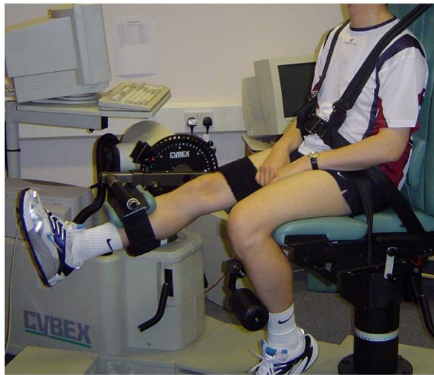
Figure 1.10: Isokinetic dynamometer used for muscle strength assessments[49]
