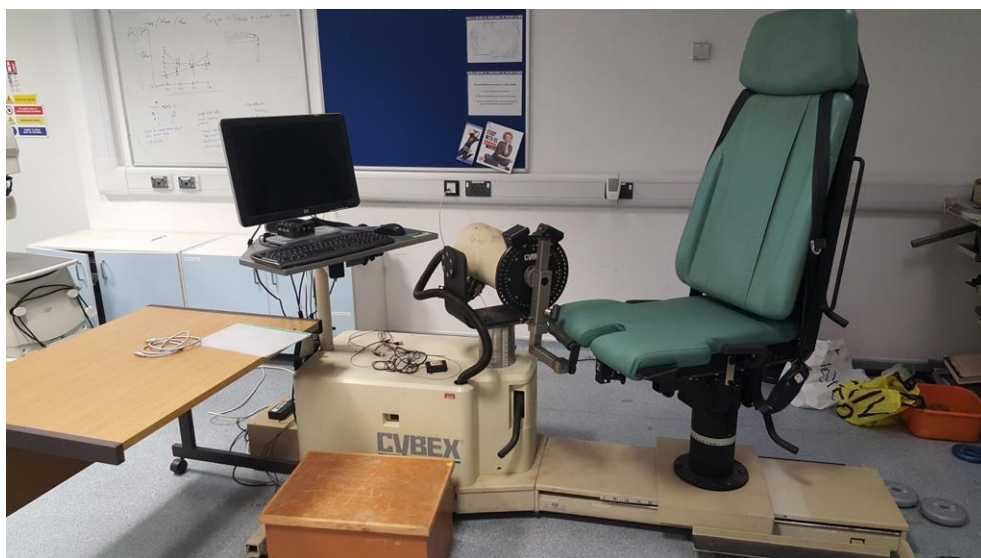
Figure 4.1: Cybex dynamometer used to measure knee torques
