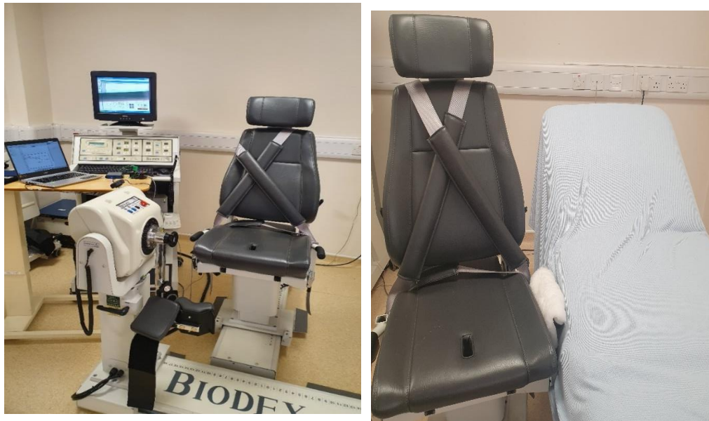
Figure 5.2: Left: setting for the dynamometry session to measure ES-induced knee torques. Right: Set-up used for participants to transfer from the height-adjustable plinth to the dynamometer chair
