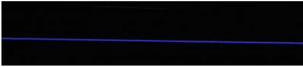
Figure 4-9: Visual appearance of corona discharge in the case of positive dc energisation.
