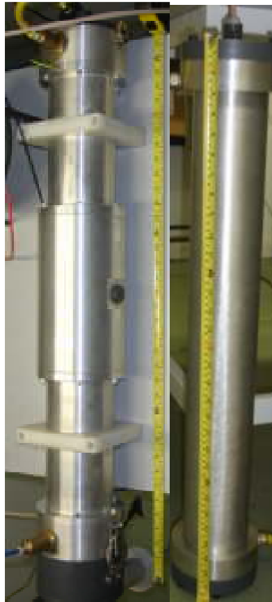
Figure 5-1: Scaled-up, double stage precipitation reactor. To the left the first (energisation) stage and to the right the second (deflection and collection of charged particles) one.
