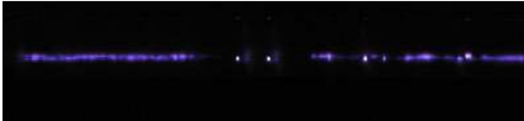
Figure 4-10: Visual appearance of corona discharge in the case of negative dc energisation.
