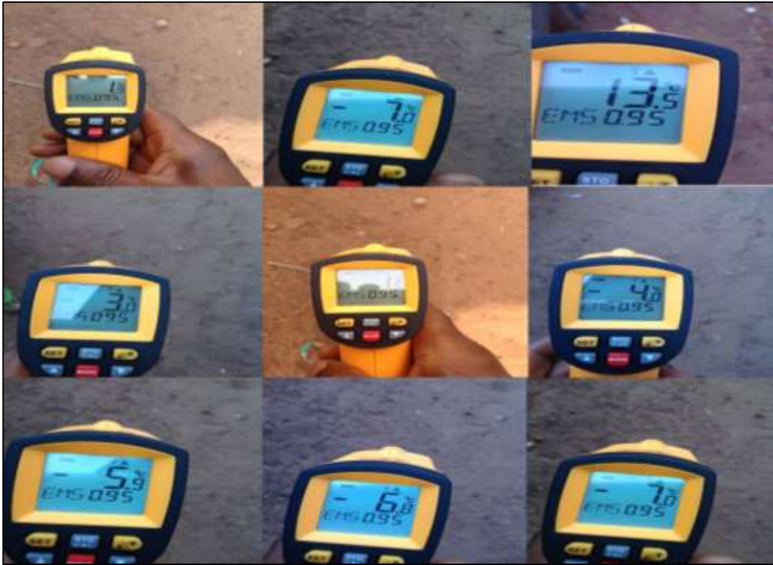
Figure 4. 12 Sky Temperature readings under various sky conditions using a Digital Handheld Laser Infrared Thermometer
