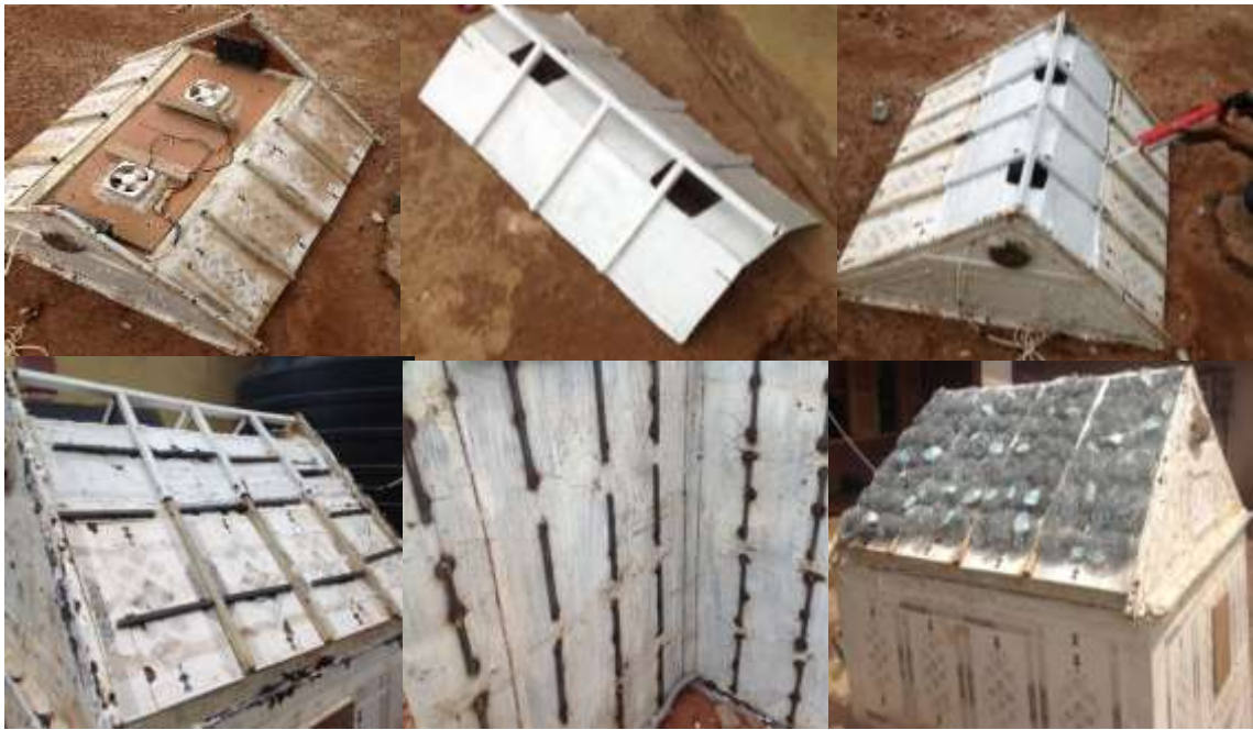
Figure 5. 49 Reconstruction of the roof system to induce turbulent air flow pattern
