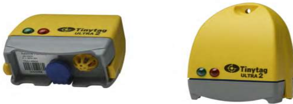
Figure 4. 3 Tinytag Ultra 2 Temperature/Relative Humidity Logger (-25 to +85°C, 0 to 95% RH)
