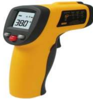
Figure 4. 5 Digital Handheld Laser Infrared Thermometer. Temperature range: -32°C to 1150°C, Accuracy: \pm 1.5\% or \pm 1.5^\circ\text{C} , Spot Ratio: 20:1, Emissivity: 0.1 to 1.00 adjustable, Resolution: 0.1°C, Response Time: 500ms, Wavelength: 8-14 \mu\text{m} .
