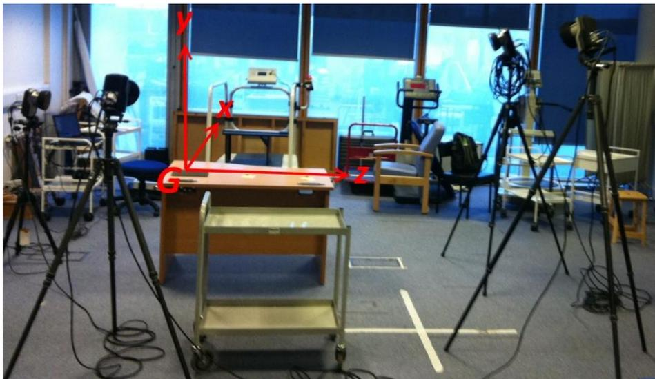
Figure 9.3: Qualisys video motion capture setup. The global reference frame (G) as defined by the Qualisys system is shown in red.
