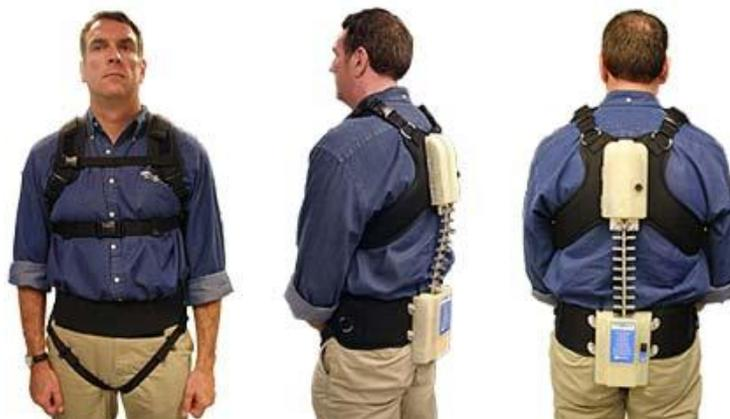
**Figure 2.13: The Lumbar Motion Monitor: a tri-axial goniometer developed at Ohio State University. (<http://www.nexgenergo.com/ergonomics/lumbarmm.html#Sec2>)**
