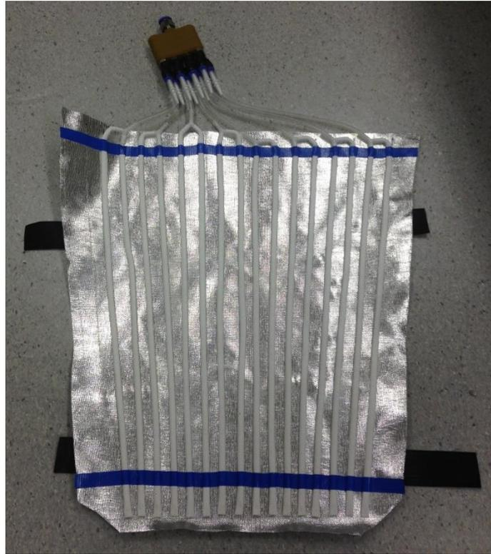
*Figure 4-9: Arrangement of tubes on 3<sup>rd</sup> iteration*
