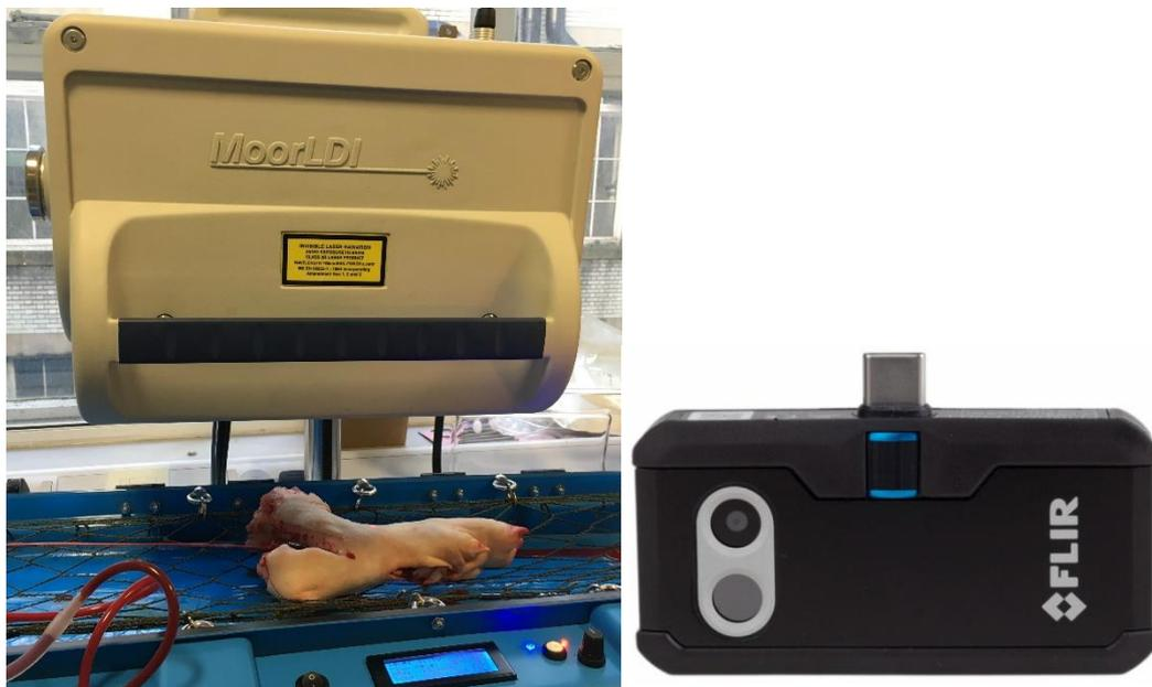
*Figure 6-2: Moor LDI imager taking an LDI scan and FLIR One Pro thermal camera used for thermal imaging. Images taken every 15 minutes during perfusion.*
