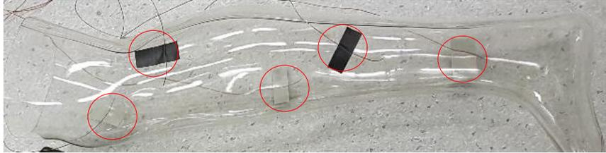
Figure 4-7: Location of the defined thermocouple positions on the mannequin limb
