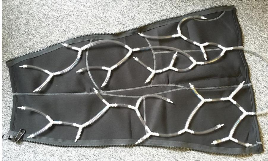
*Figure 4-29: Arrangement of tubes and outlets in the seventh iteration of cooling sock*
