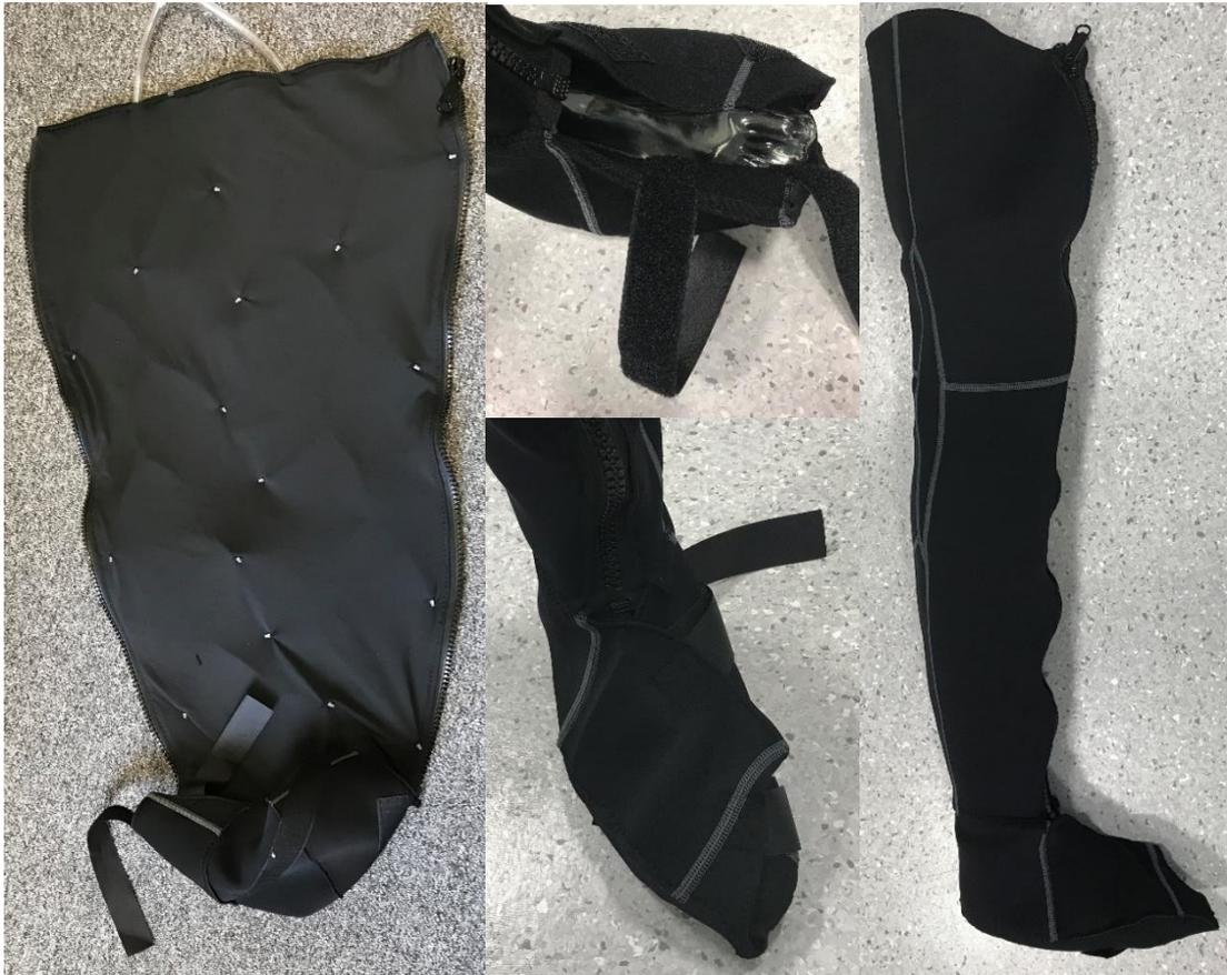
*Figure 4-31: Eight iteration of cooling sock. Both open and closed as well as close ups of foot covering mechanism*
