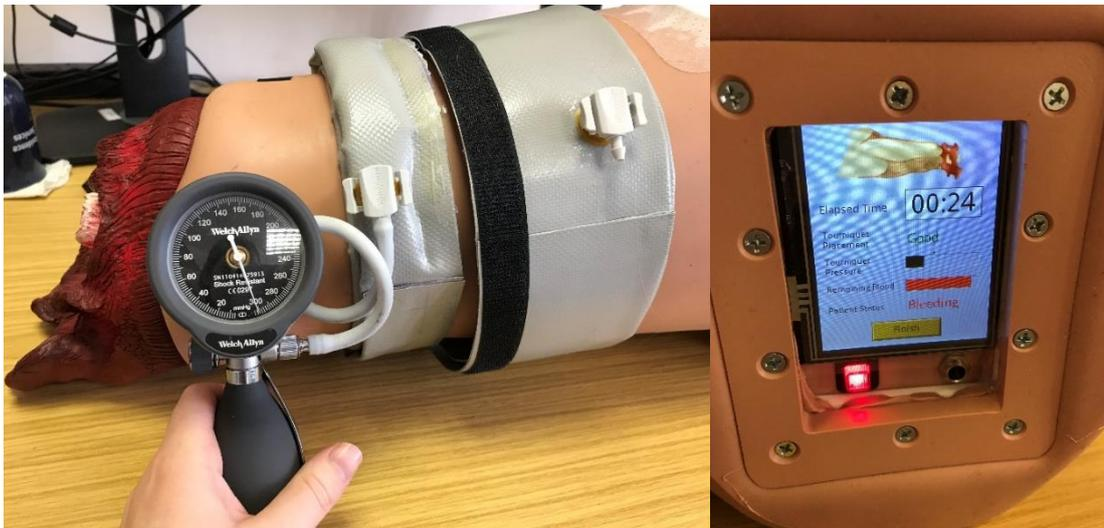
Figure 3-13: Testing of tourniquet iteration 6 on the HapMed and a close-up of the results screen
