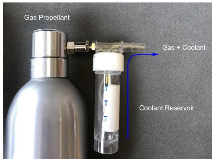
Figure 4-28: Gas and coolant distribution mechanism
