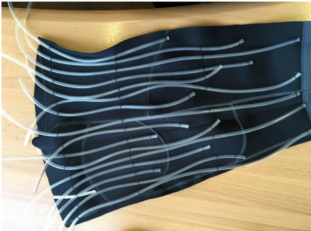
*Figure 4-25: Layout of non-porous tubing for smaller version of 6<sup>th</sup> iteration*
