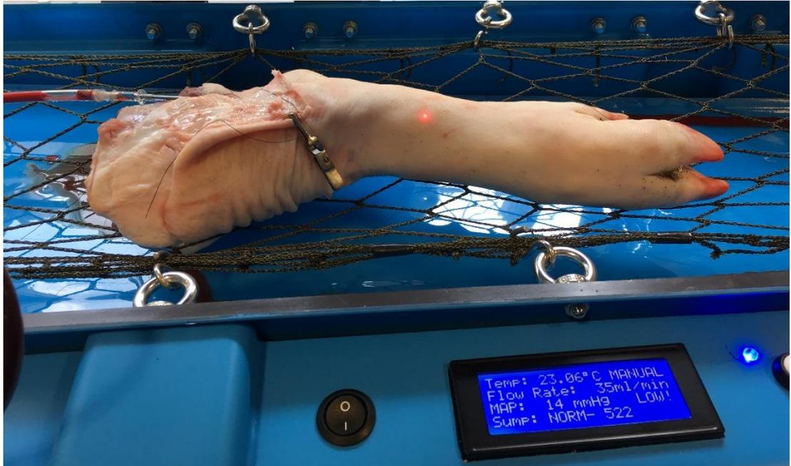
Figure 6-3: Disarticulated porcine limb being perfused in the LSS with mean arterial pressure and flow rate displayed on screen. Red dot is the LDI scan being performed. Cannula is filled with primer fluid
