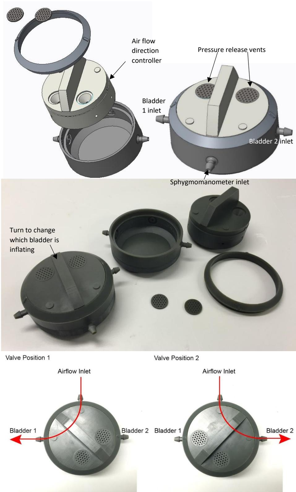
Figure 3-1: CAD drawing and 3D printed dual way valve with inflation mechanism demonstrated
