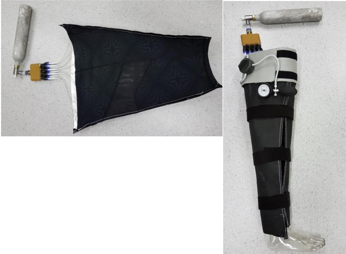
Figure 4-6: 2<sup>nd</sup> iteration of cooling sock both open and closed around the mannequin leg.
