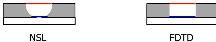
Figure 3.10 – Cross-section of Ag nanohole to illustrate difference in structure between NSL fabricated hole and FDTD simulated hole. The red line represents the diameter at the surface of the hole whilst the blue line represents the diameter at the base of the hole.
