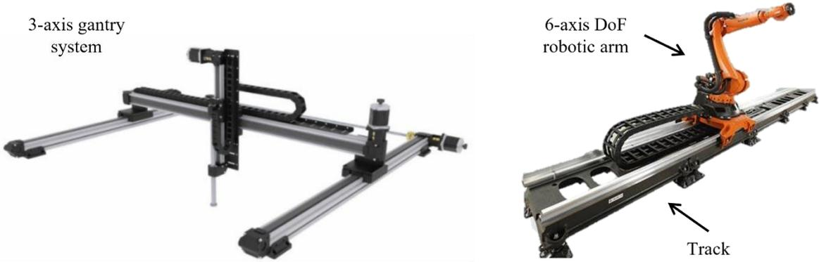
*Figure 2.12 Axial manipulators suitable for automated NDE delivery*
