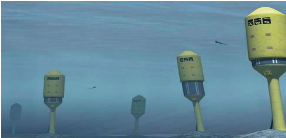
Figure 2.6: submerged pressure differential device: the Archimedes Wave Swing. Figure is taken from Drew et al. (2009).
