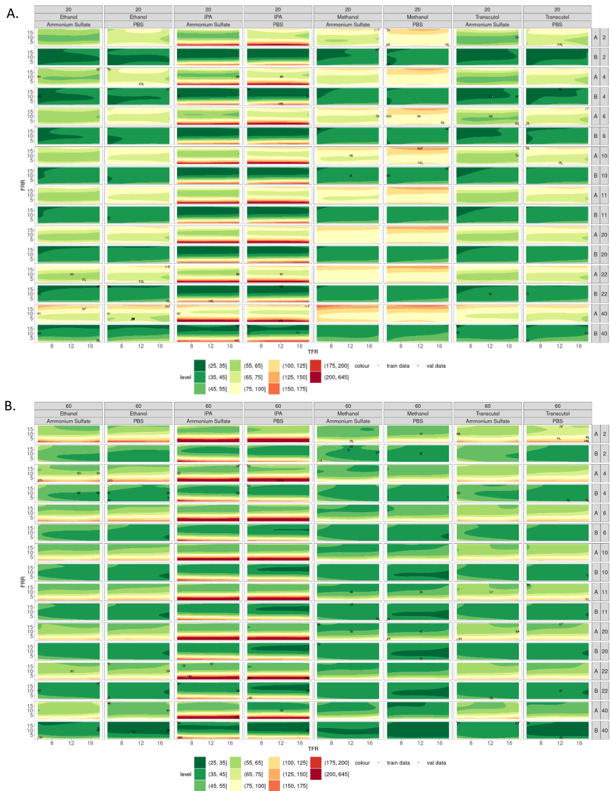
Figure 3.5: Contour plots of particle size produced across all the variables tested. A) Liposomes produced at 20°C from lipid A (DSPC) and lipid B (DOPC) at concentrations of 2 – 40 mg/mL. B) Liposomes produced at 60°C from lipid A (DSPC) and lipid B (DOPC) at concentrations of 2 – 40 mg/mL where smaller liposomes are shown in green and larger liposomes are shown in red.
