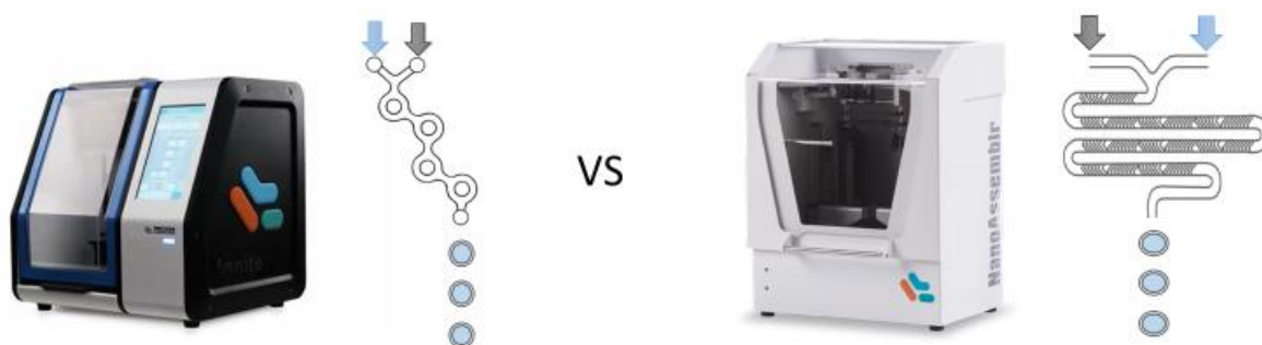
Figure 2.18: Micromixer designs. A) Toroidal mixer that was used on the Ignite vs B) Staggered Herringbone mixer used on the Benchtop. Adapted from https://www.cytivalifesciences.com
