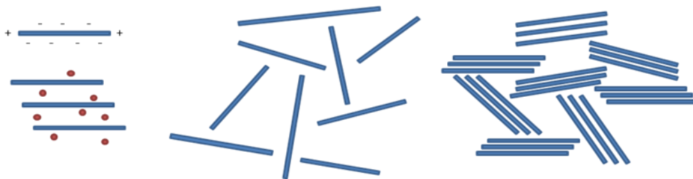
Figure 1.2 Illustration of an individual platelet with surface and edge charges, an individual tactoid with hydrated counter-ions, card-house structure and book-house structure.
