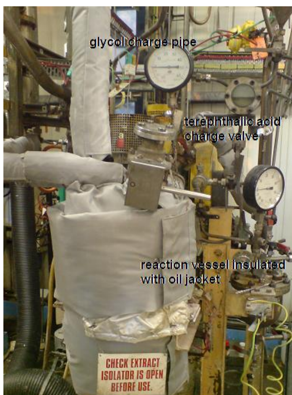
Figure 3.4 Photograph of the 7 kg (5 gallon) batch reactor used to prepare the polymer and polymer composite chip.
