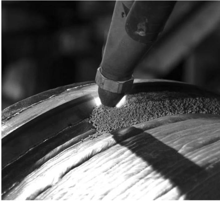
Figure 2.2: SAW welding, with weld torch surrounded by granular flux [42]
