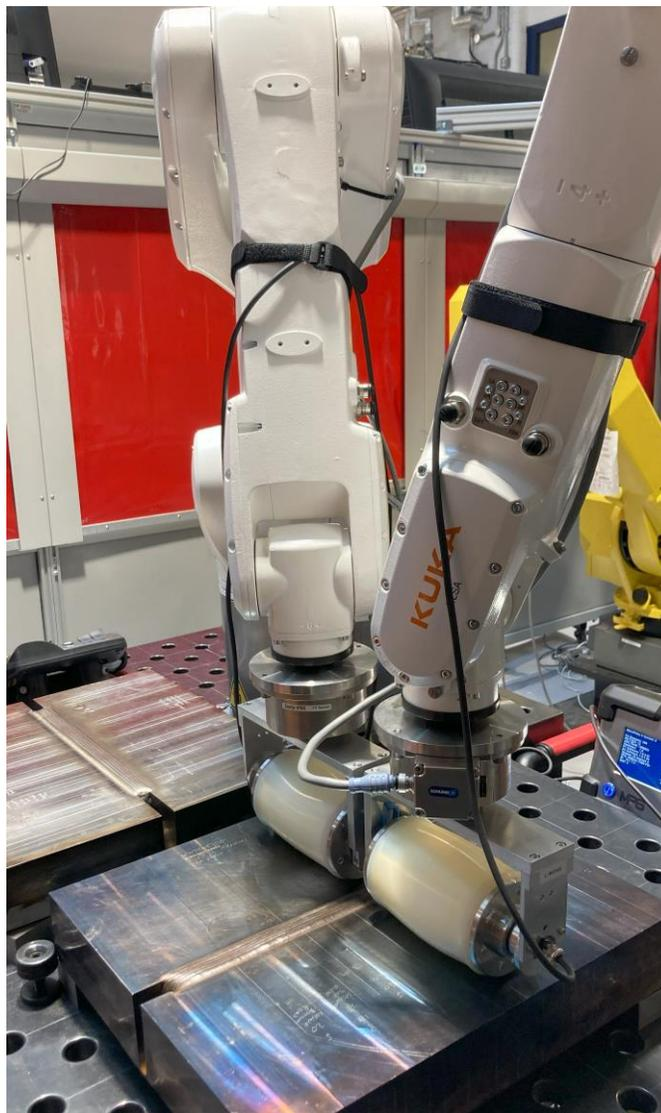
Figure 6.3: Tandem phased array setup on a narrow gap weld using two robotic manipulators with dry-coupled high-temperature roller probes
