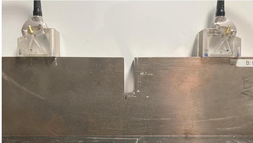
Figure 4.5: Sample PNG4 with dual-array setup, highlighting simulated 70.0 mm weld fill height and 65.0 mm EDM notch height.
