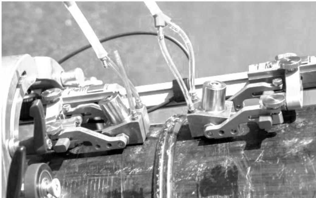
Figure 2.16: Orbital TOFD scanner [112]
