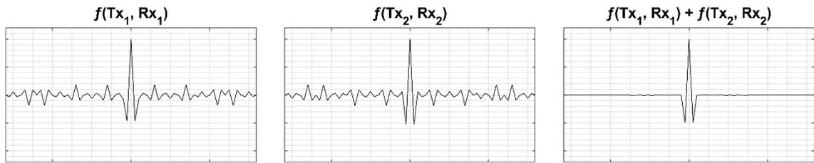
Figure 5.2: Demonstration of sidelobe suppression by the sum of two complimentary Golay functions, resulting in a single main lobe
