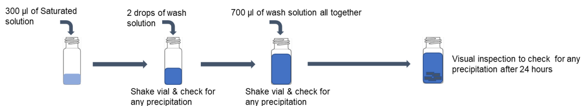
Figure 2-2: Glass vial precipitation detection method
