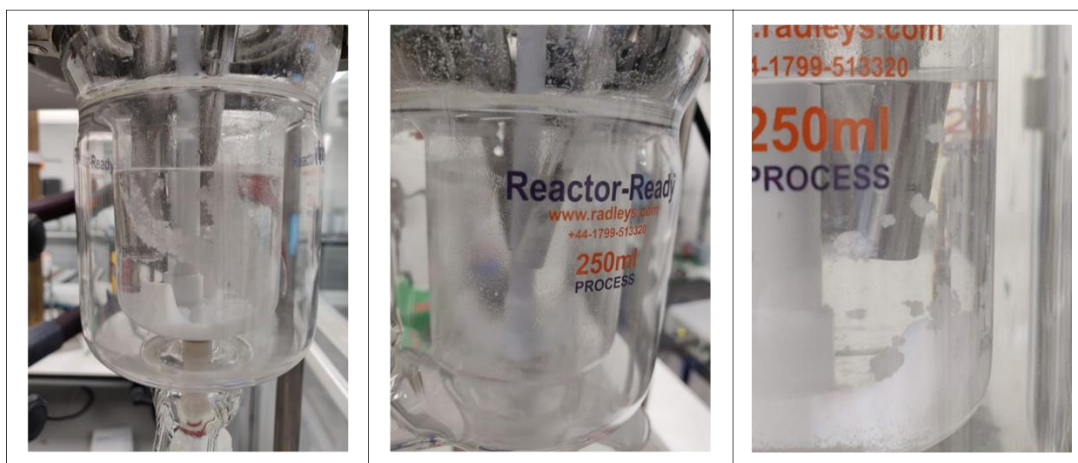
Figure 4-23: Images showing PCM API stuck to the wall of the vessel and the probe at the end of analysis.
