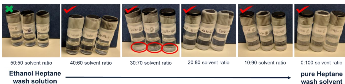
Figure 2-4: Ethanol - n-heptane glass vial precipitation qualitative test
