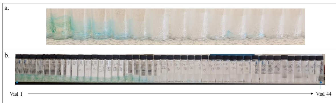
Figure 3-4: a.) Close-up of a few dried filtrate vials showing presence of precipitated material. b.) Collected filtrate vials from experiment 15 showing gradual blue dye impurity removal from the system
