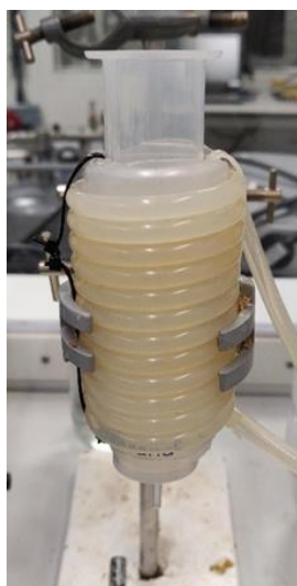
Figure 5-2: Cooling jacket used for biotage filter tube
