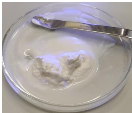
Figure 4-6: Filtered and washed crystalline PCM API cake which is not deliquored properly
