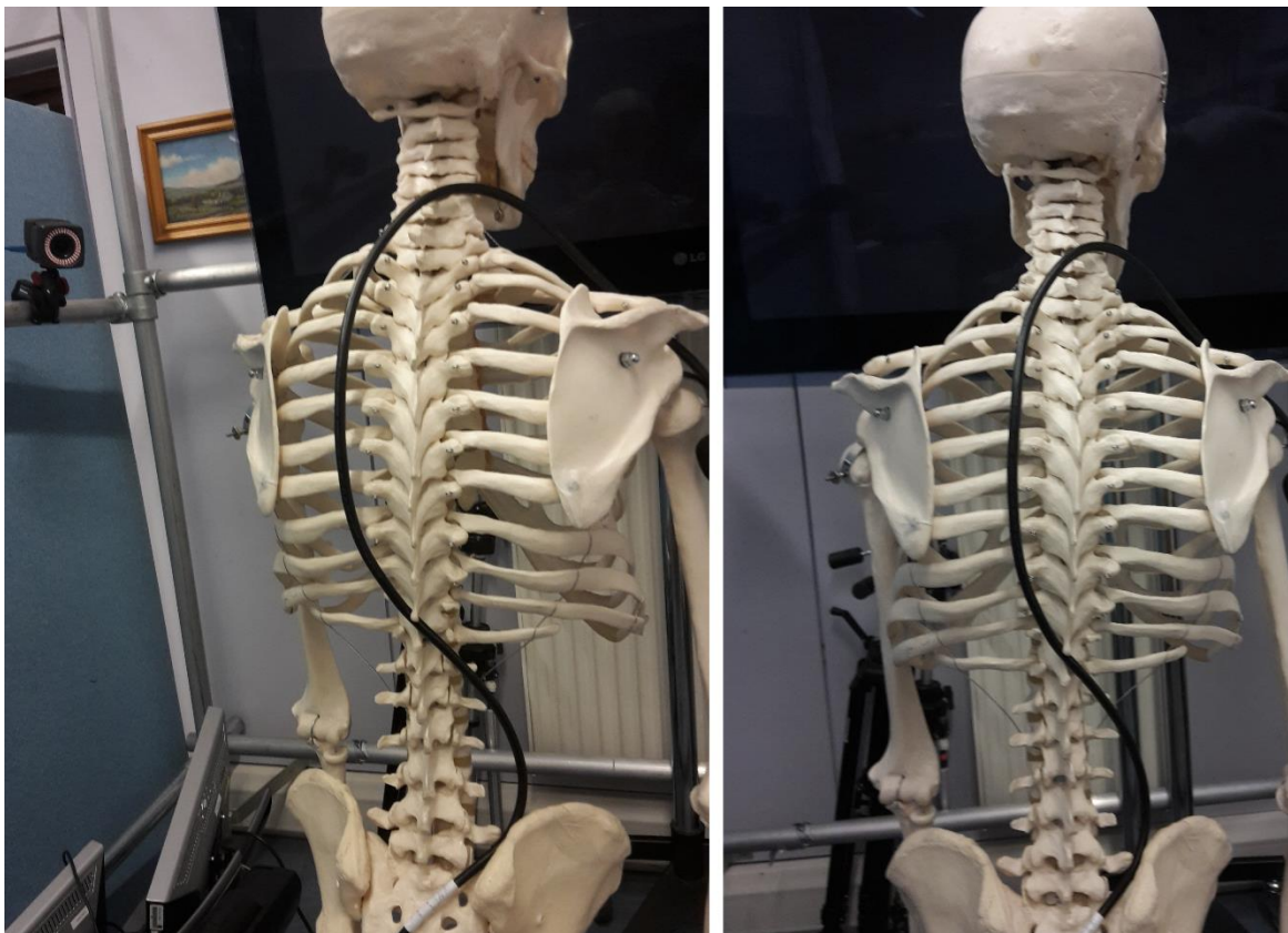
Figure 7.1.1: S-shaped cable at the back of the skeleton, mimicking geometry of patients with scoliosis
