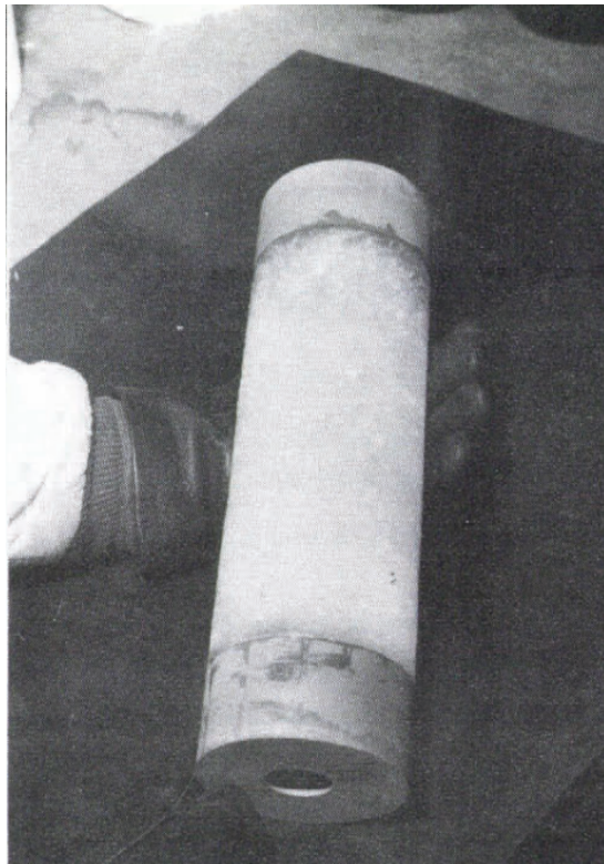
Figure 2.8: Saline-ice specimen with end caps, Cole et al. (1985)
