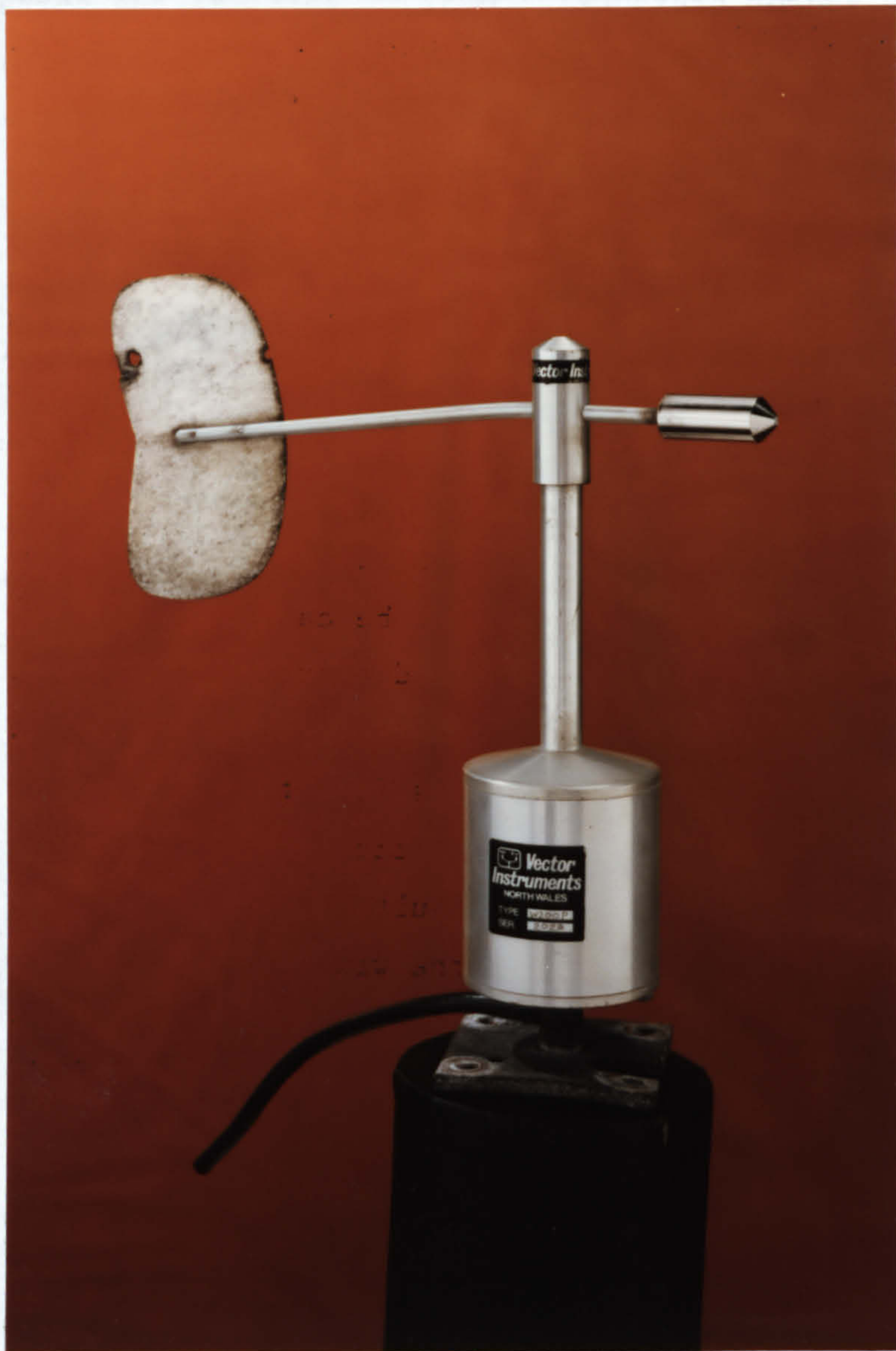
Figure 5.11 : Lightning damaged wind vane
